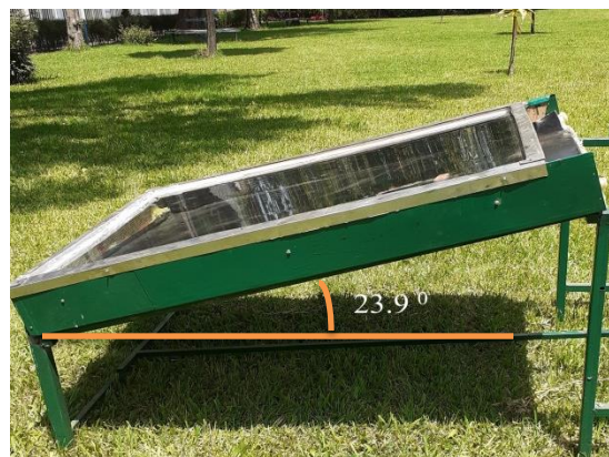
Figure 4.12- Tilt angle of the solar collector
