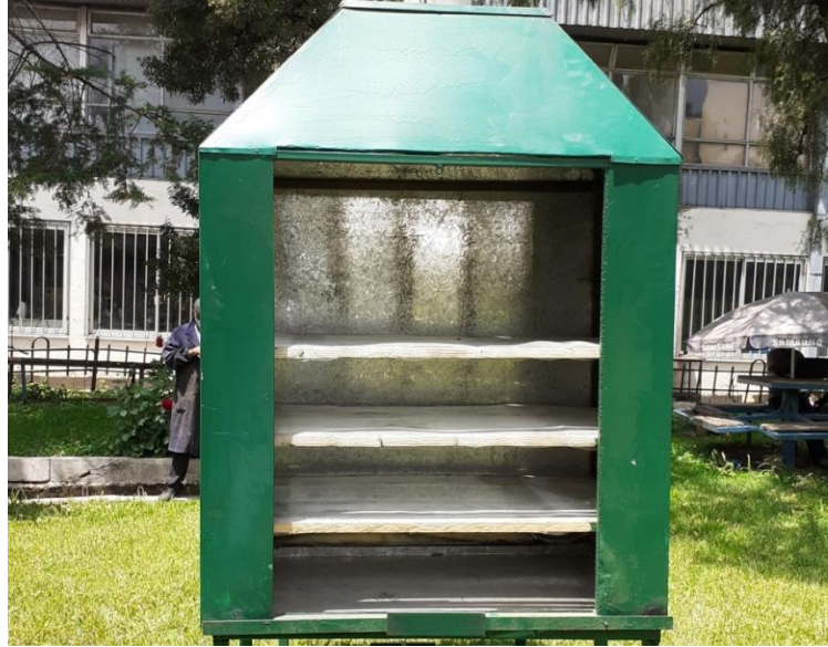
Figure 4.9- Drying chamber of the solar tea dryer
