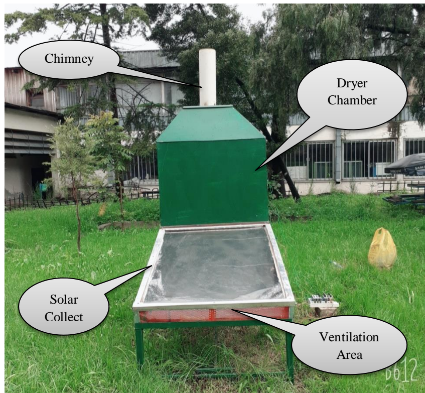
Figure 5.1- Setup of the solar dryer
