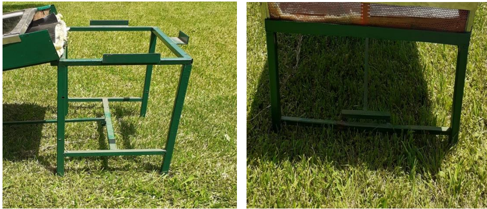
Figure 4.11- Back and front leg of the solar tea dryer
