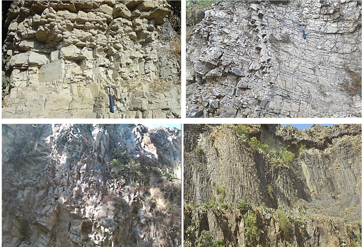
Plate 2.3 selected joint sets with different orientation in the study area
