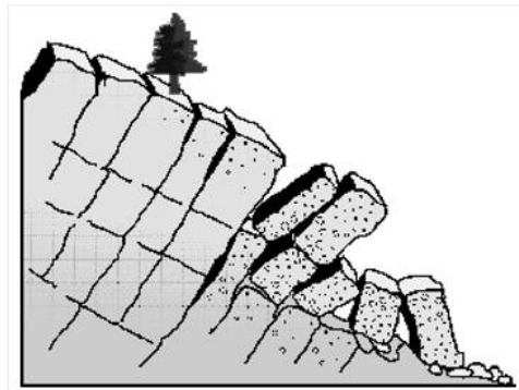
Fig. 3.12 Toppling mode of failure (Deep et al., 2014)
