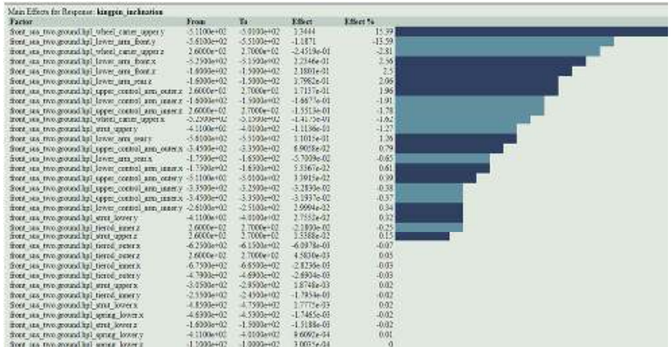
Figure 5. 33 Pareto charts for kingpin inclination angle
