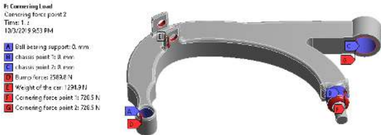
Figure 3. 10 Load histories in a cornering maneuver
