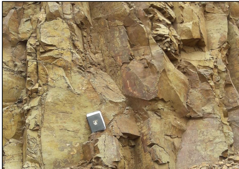
Fig. 3.5: Glassy rhyolite outcrop which is strongly fractured and jointed with vertical to sub-vertical joints at a quarry site (0601123 E: 1103127 N).
