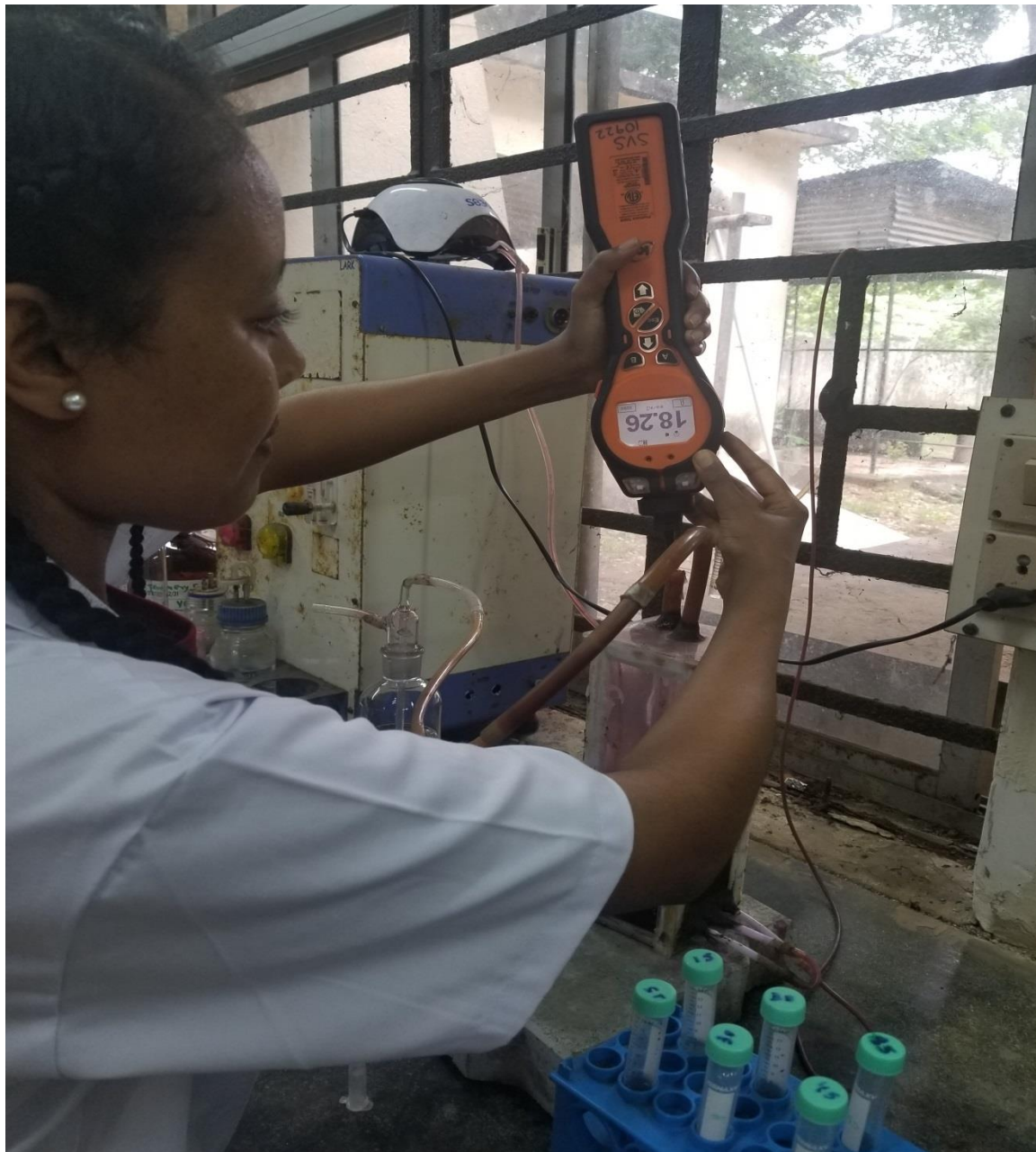
Figure 3. 4: Detection of VOC using Photo Ionization Detector
