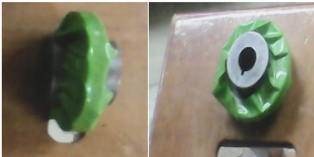
Figure 3.10: Method of plastics application on the rail side wheel surface
