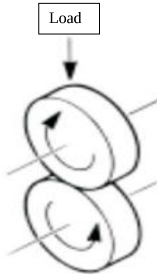
Figure 1.2: contact mode of the twin disks [5]
