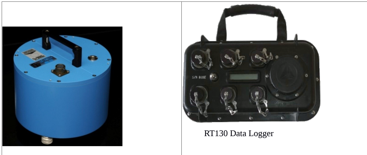
Figure 5.4 the seismic sensor and data logger deployed in the new permanent seismic station at Wolmera. The sensor is short period Le-3d/5sec, with Refraction technology RT130 data logger.
