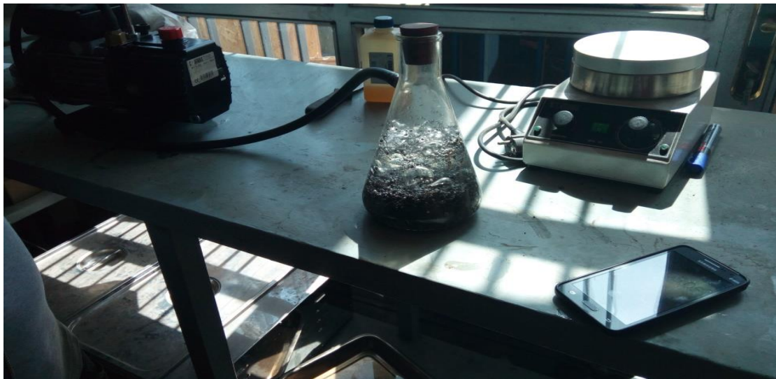
Fig. 3. 12 Vacuum application for saturated sample
