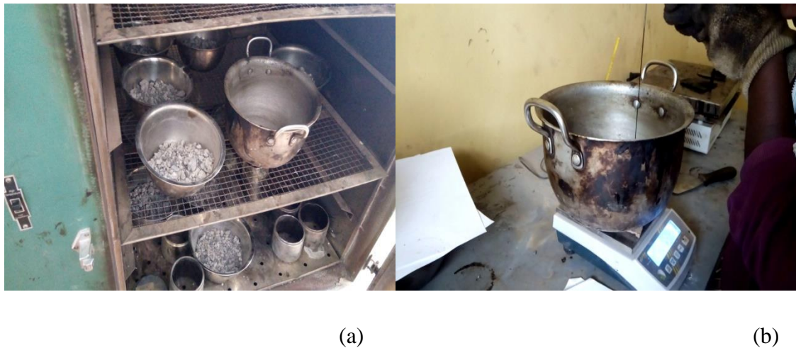
Fig. 3. 7 aggregate and mixing tools heating (a) & pouring of bitumen to aggregate (b)
