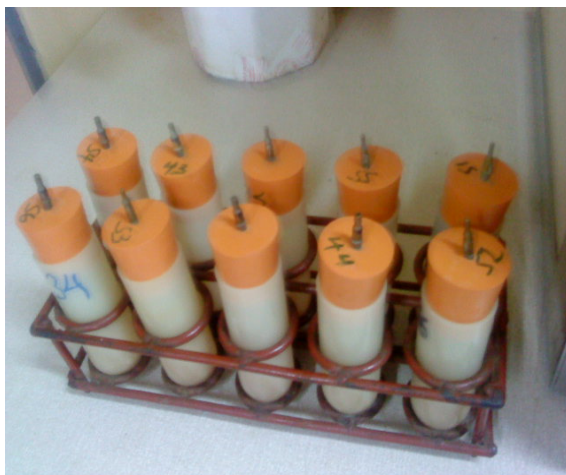
Figure D-1 Flask where the rumen fluid and plus P.Juliflora placed and sealed to create anaerobic environment inside the flask
