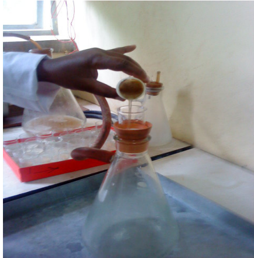
Figure D-2 filtration of the residue from the digested fluid
