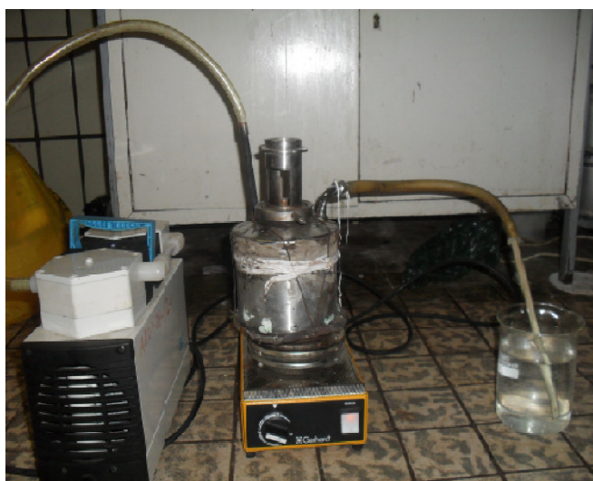
Figure B-2 Laboratory set for preparation of Sulphuric acid from sulfur powder
