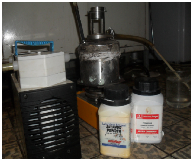
Figure B-2 Laboratory set for preparation of Sulphuric acid from sulfur powder
