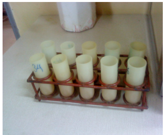
Figure D-1 Flask where the rumen fluid and plus P.Juliflora placed and sealed to create anaerobic environment inside the flask
