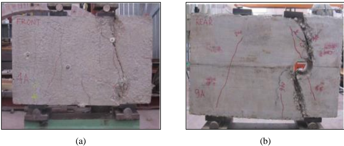
Figure 2-13 (a) Specimen without opening (b) specimen with openings with in the shear zone
