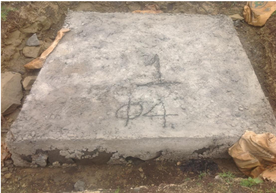
Figure 12 28 days Concrete Sample #1 (6cm thick concrete and \phi 4 wire mesh)
