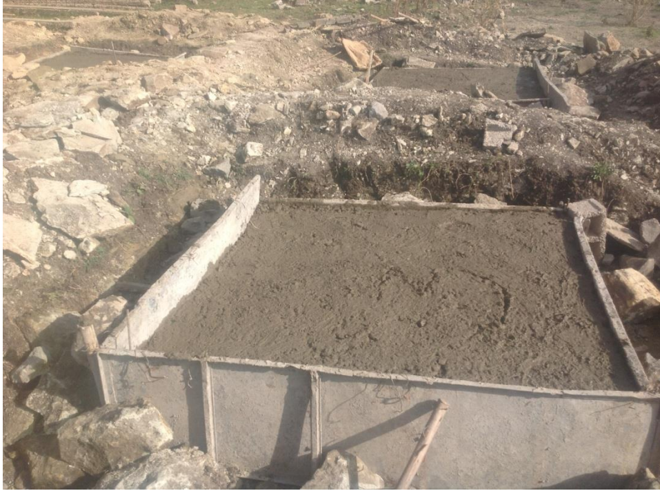
Figure 9 Fresh Concrete Cast of Sample #3 (8cm concrete thickness with no wire mesh)
