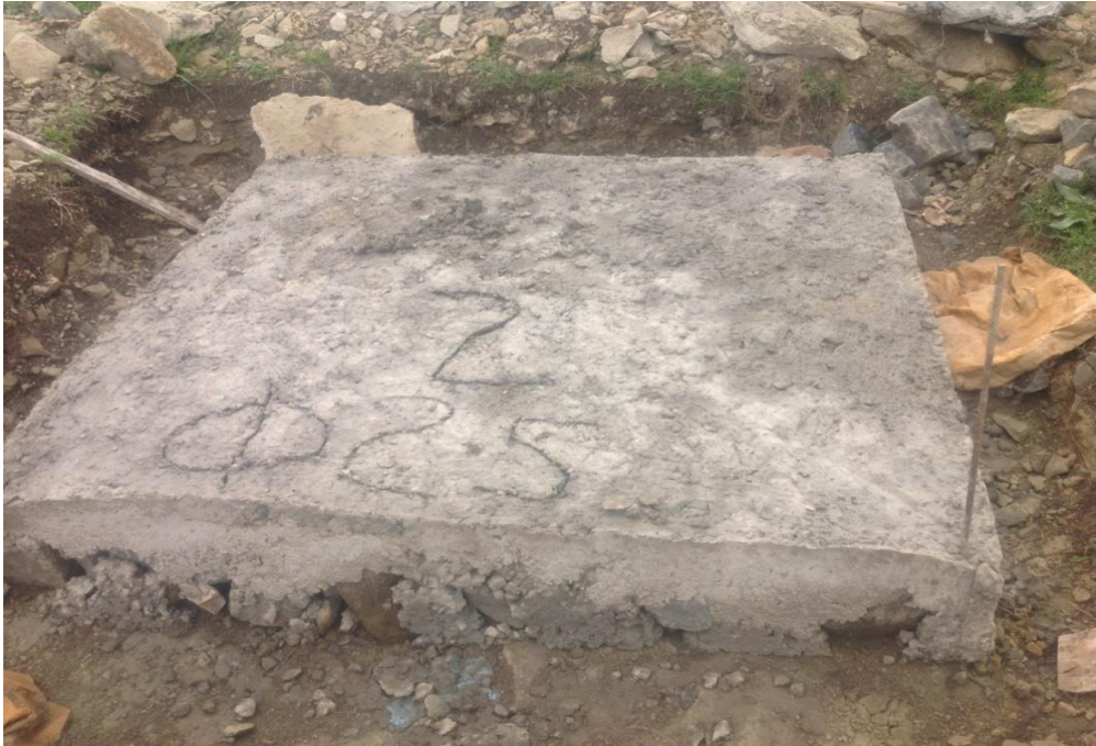
Figure 13 28 days Concrete Sample #2 (6cm thick concrete and \phi 2.5 wire mesh)
