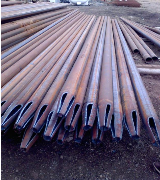
Figure 7 Pipes for umbrella arch purpose
