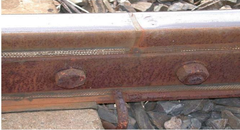
Figure 1.5: Unsymmetrically suspended IRJ
