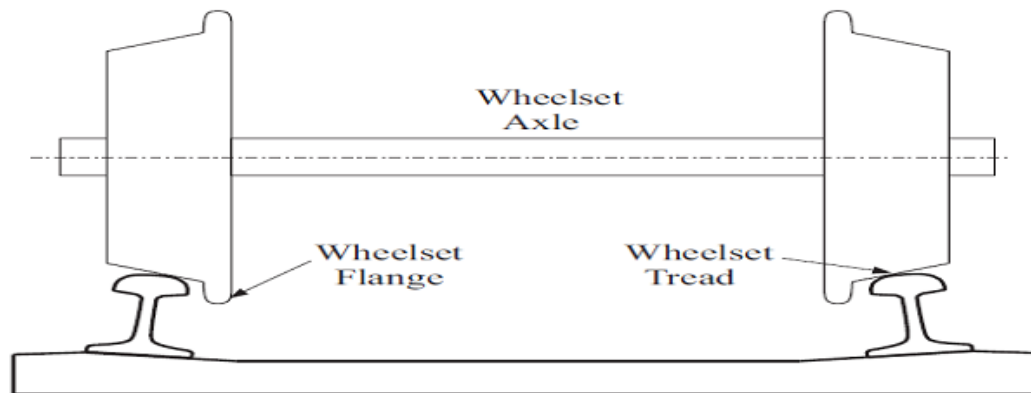
Figure1.1: Assembly of rail wheel axle.
