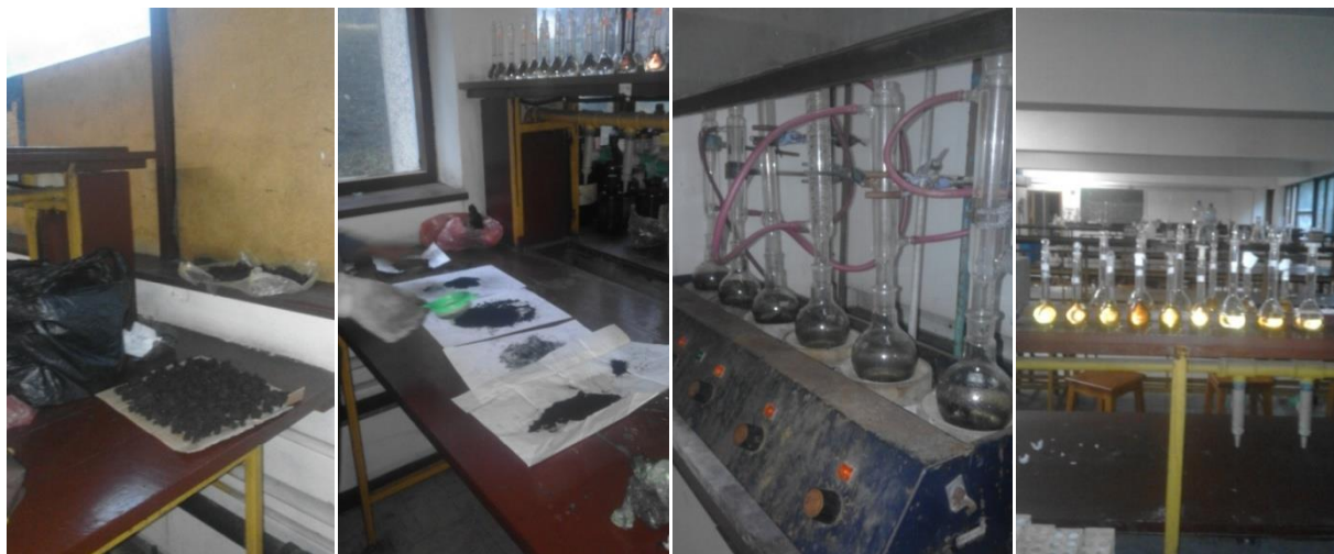
Figure 4 Soil samples, Kjeldahl digestion apparatus and digested solution
