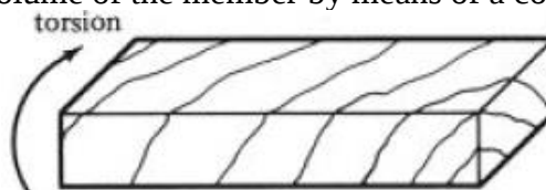
Fig. 4.39: Illustration of torsional cracks
