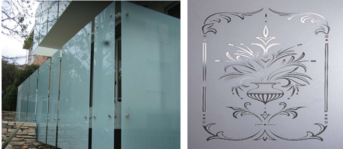
Figure 2-43: Sandblasted glass (on the left-hand side) and acid-etched glass (on the right-hand side)
