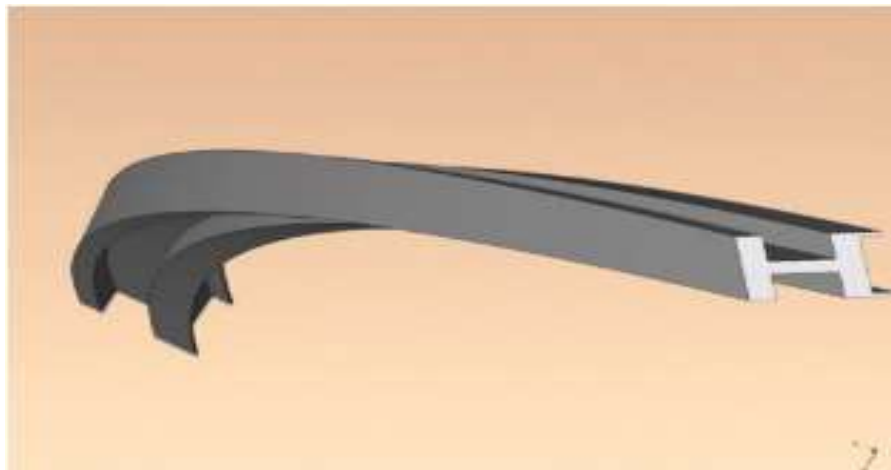
Figure 3-12: Twisted Aluminium profile for twisted curtain wall (Vollers, 2004)
