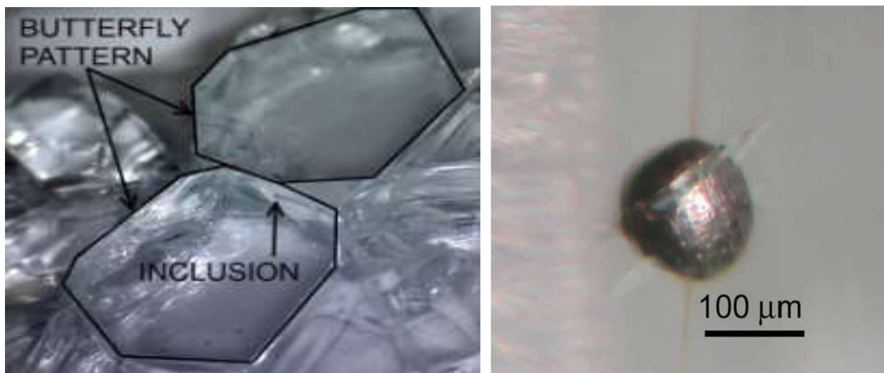
Figure 2-51: Nickel sulfide inclusion
