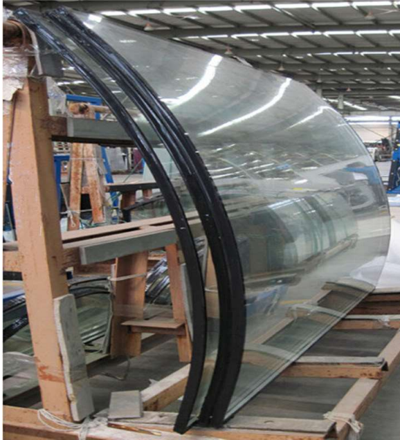
Figure 3-13: Single curved IGU glass
