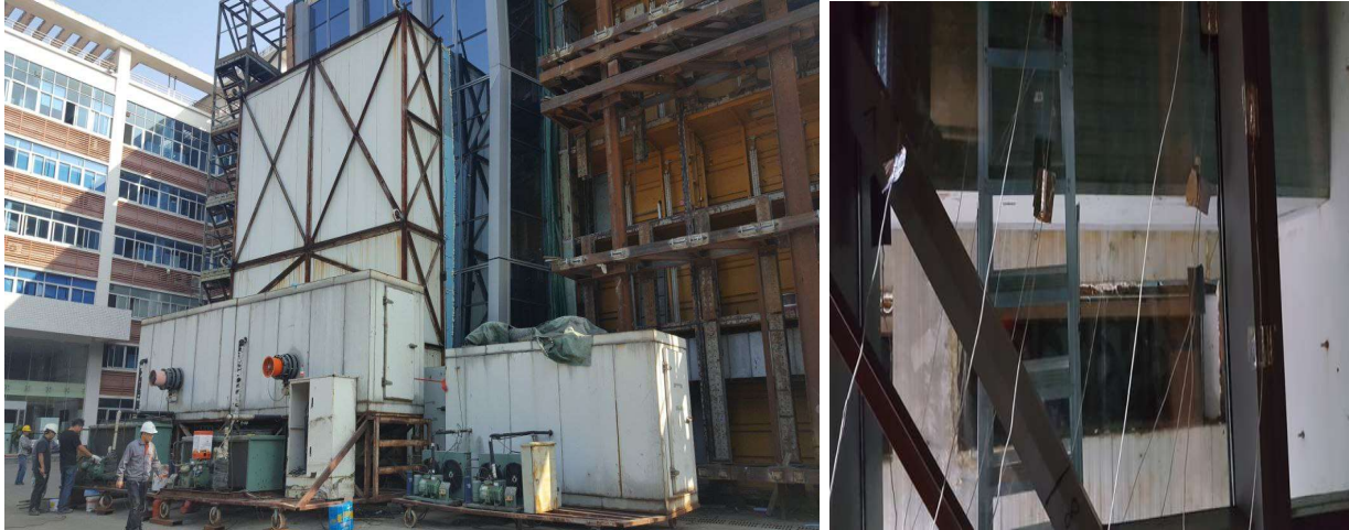
Figure 5-15: Thermal Cycling Test setup
