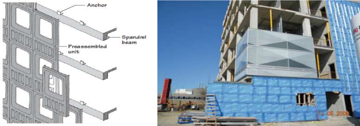
Figure 2-7: Panel system curtain wall
