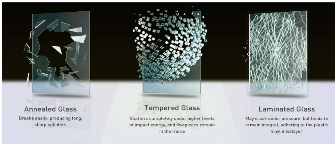
Figure 2-39: Breakage pattern of Annealed, tempered, and laminated glass
