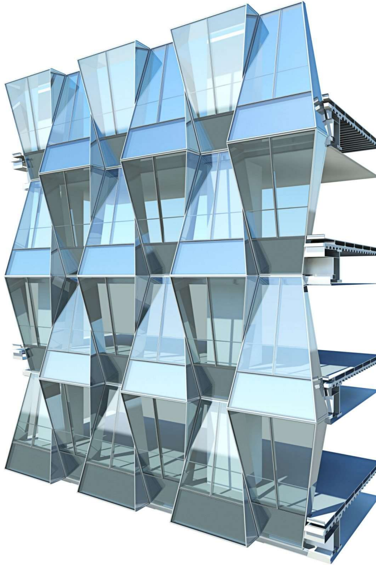
Figure 3-8: Double sheared complex unitized curtain wall
