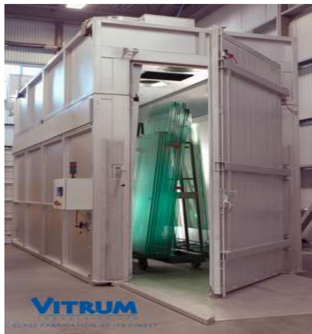
Figure 2-52: Heat-soak testing oven
