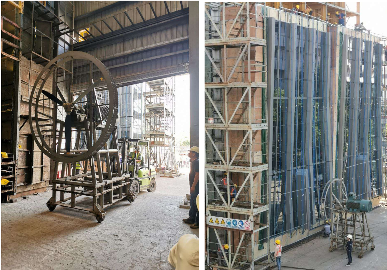
Figure 5-14: Aircraft propeller for dynamic water penetration test
