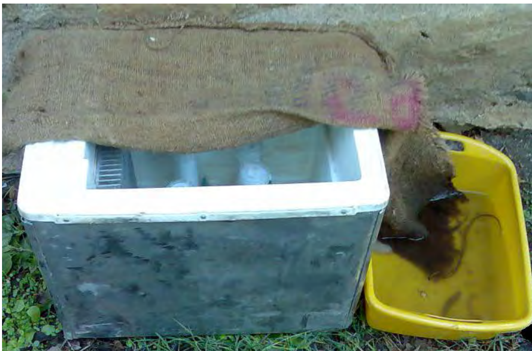
Plate 5. The cool box used in the field containing the exposure tubes and holding tubes.
