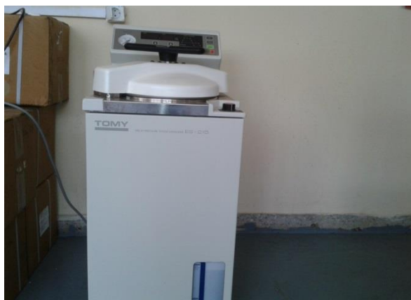
Figure 3.4: Autoclave apparatus for fleshed waste hydrolysis
