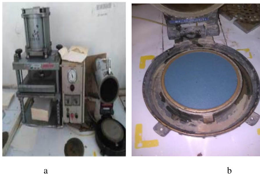
Figure .3.4: Sheet forming and pressing machine (a) Pressed blende waste beer label sheet (b)
