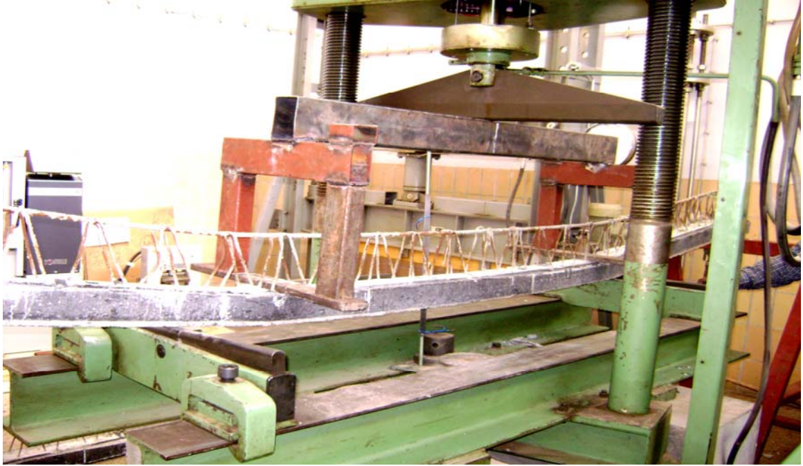
Fig.2.1 Bending Test Setup
