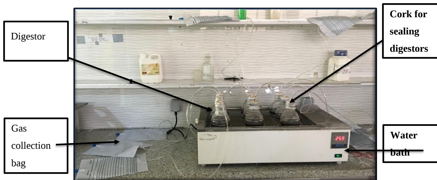
Figure 3.2 Anaerobic digestion setup
