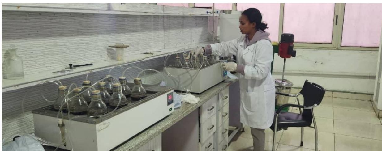
(f) Anaerobic digester setup and temperature regulation
