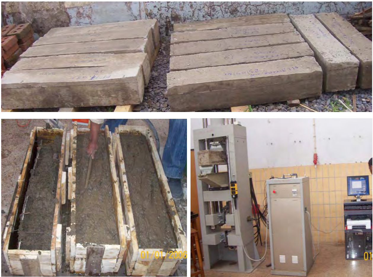
Figure 3.9 Flexural Test Specimens and Set Up
