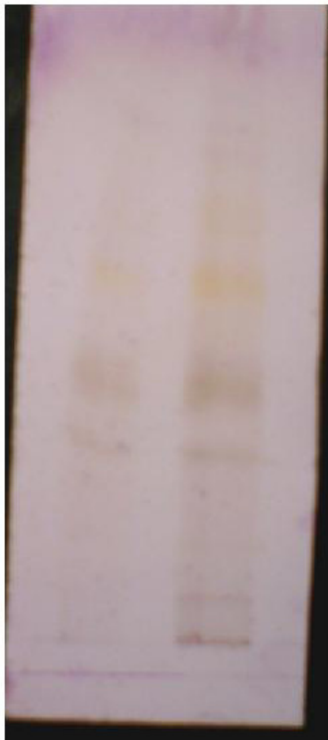
Figure 3.3: Thin Layer Chromatogram of the methanol and total extracts of M. lanceolata after treatment with vanillin-sulphuric acid spray reagent.
