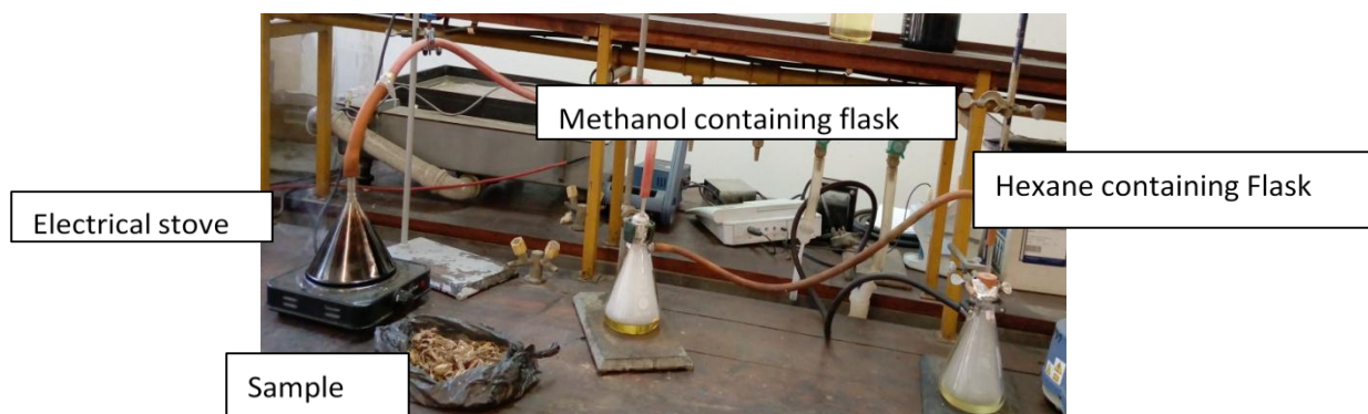
Figure 6. Set up of smoke trapping system
