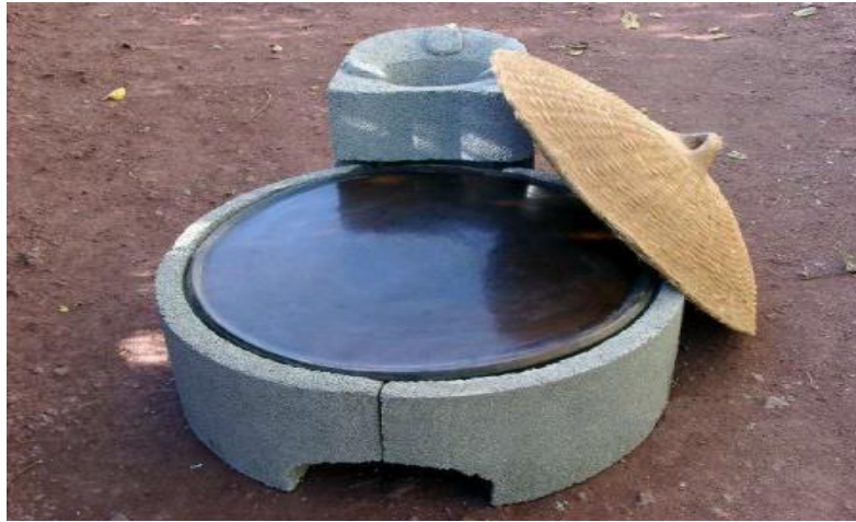
Figure 6: Mirt Injera Baking Stove (Gulilat & Girma, 2011)
