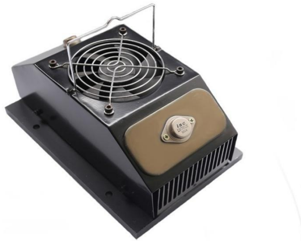
Figure 31: Packaged TEG module ("Stove Top TEG,")
