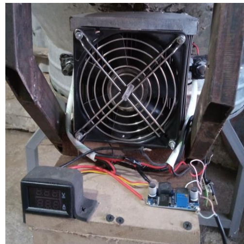
Figure 39: TEG Integration setup
