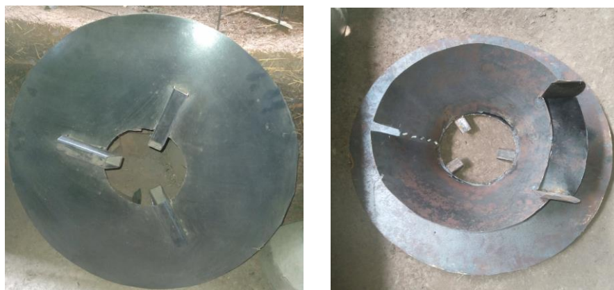
Figure 35: Manufacturing of cooking combustion chamber assembly
