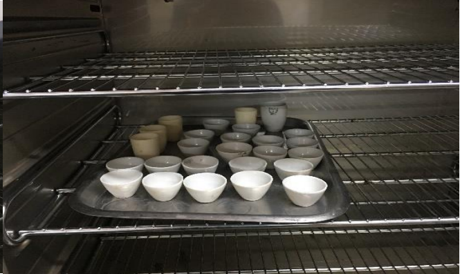
sample in oven for moisture content determination Crucible pre drying for ash determination
