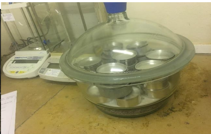
box pre drying in oven and boxes in desiccator for moisture content left to right
