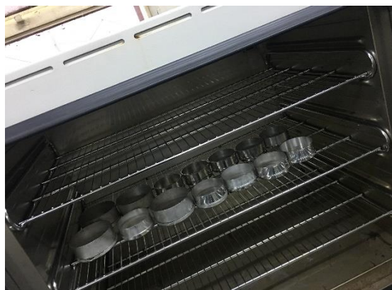
box pre drying in oven and boxes in desiccator for moisture content left to right
