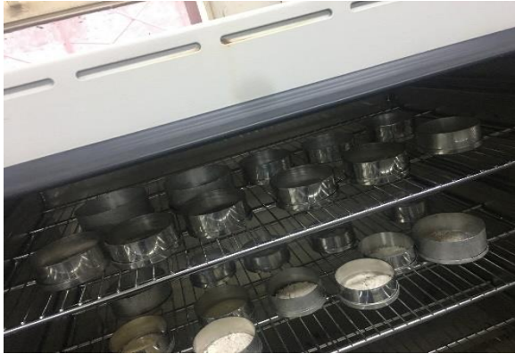
sample in oven for moisture content determination Crucible pre drying for ash determination
