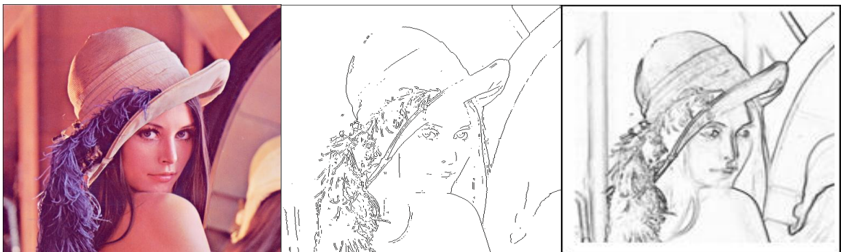
Figure 2.7. Results of edge detection applied to color test image of Lena. Original color image (left), gray scale-based edge output (middle) and result using vectorial (trinion based) approach (right).
