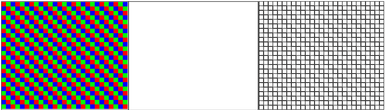
Figure 1.2 Matlab generated synthetic color image consisting of three different color squares of similar intensity in a grid pattern (left), its corresponding gray scale image (middle) and results of vector-valued (Trinion based) edge (right).
