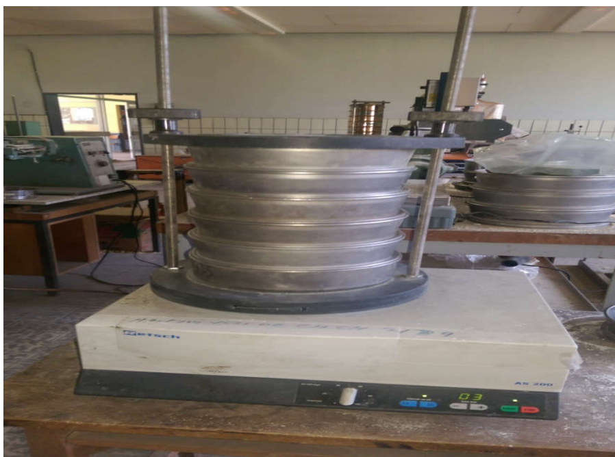
Figure F.4 vibrating shaker (Retsch) during sieves analysis of particle size.
