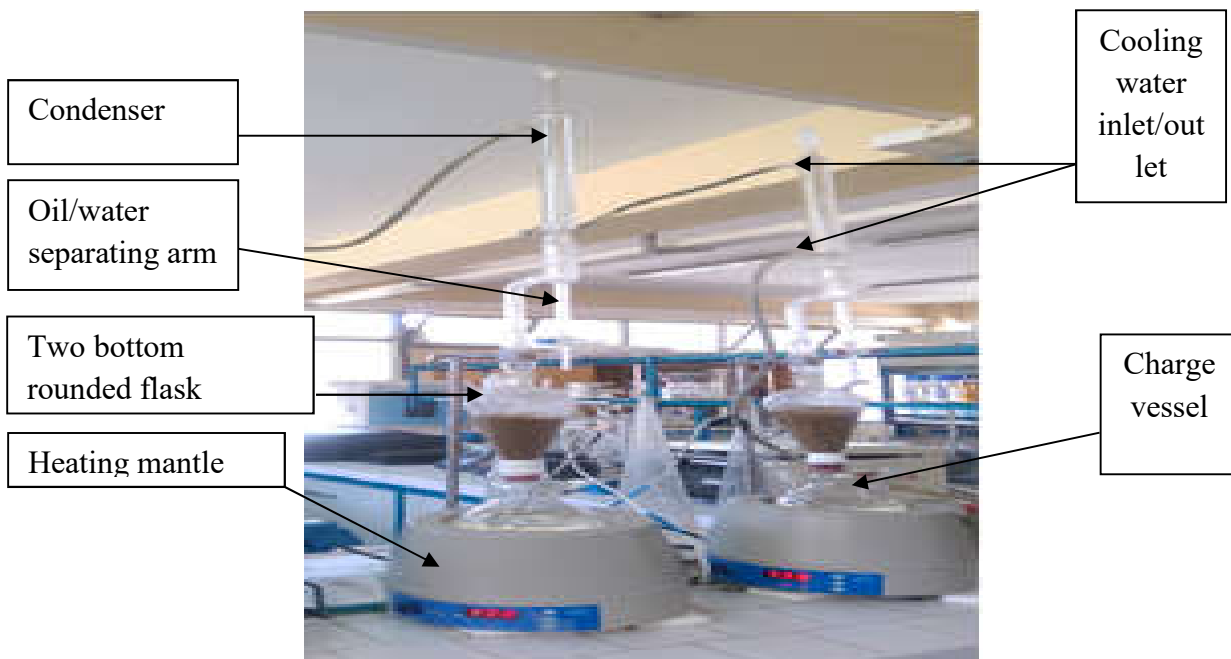
Figure 3.3 Steam distillation laboratory scale setup at LIDI, (2017).
