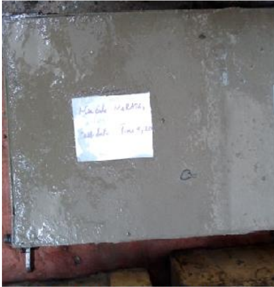
A) Mix 4 Radiation Attenuation Test Sample (75% Hematite)
