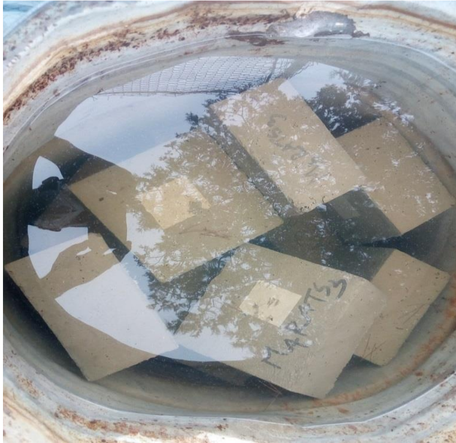
Figure 6.6.2b: Concrete Samples Cured in Water Tank
