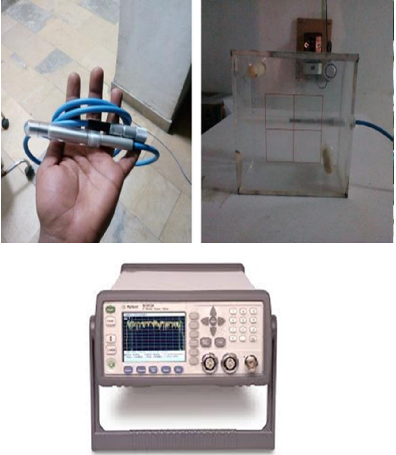
Figure 6.7.3.2e: Left-Ionization chamber, right-Ionization chamber fixed in a glass enclosure and bottom-Electrometer used to measure the current (Devices used together to measure the amount of charge produced in Air by the Cobalt-60 isotope)
