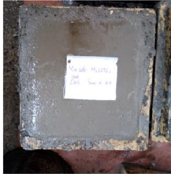
B) Mix 4 Compressive Strength Test Sample (75% Hematite)
