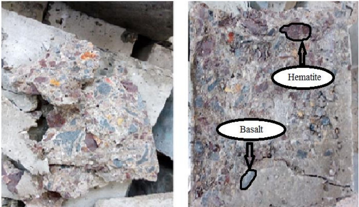
Figure 6.7.2.3b: Left side, broken sample after compressive strength test and right side, hematite and basalt aggregates are visible in broken samples after the compressive strength test
