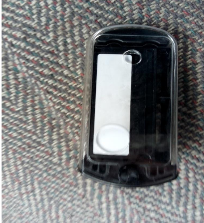
Figure A-2e: Personal Film Dosimeter which measure the Radiation intake of the researcher during the experiment
