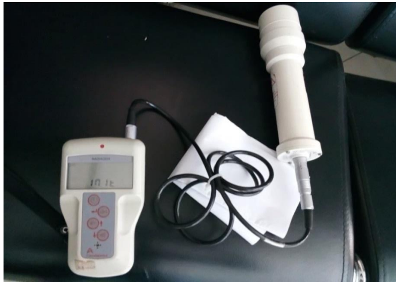
Figure 6.7.3.1a: Radiation survey meter used for assessing the maximum radiation intensity
