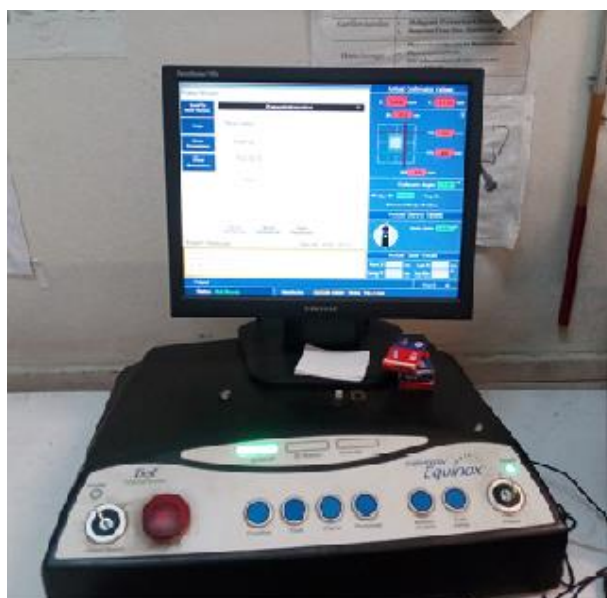
A) Co-60 Teletherapy Machine-Radiation Level and Collimator Monitor
