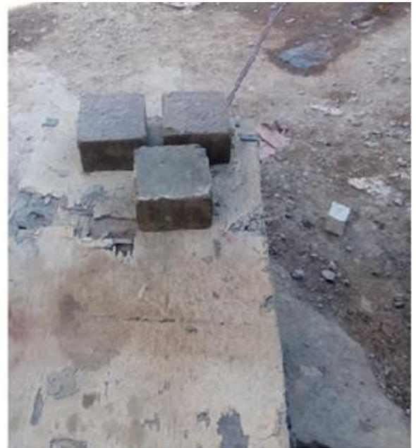
B) 200*200*100 mm Concrete Samples with 50% Hematite Aggregate
