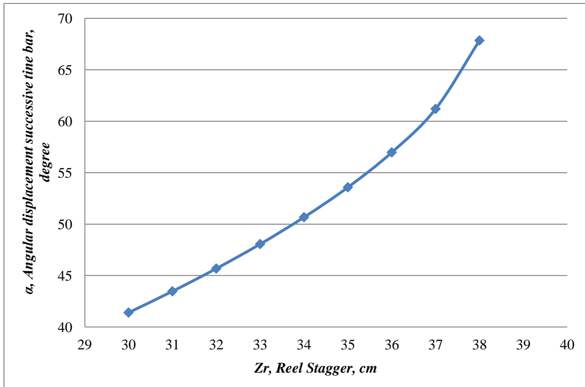
Fig. 16 Effect of reel stagger on angular displacement of successive tine bar, radius of reel R = 53 \text{ cm} and deflection angle of tef crop \varphi = 54^\circ
