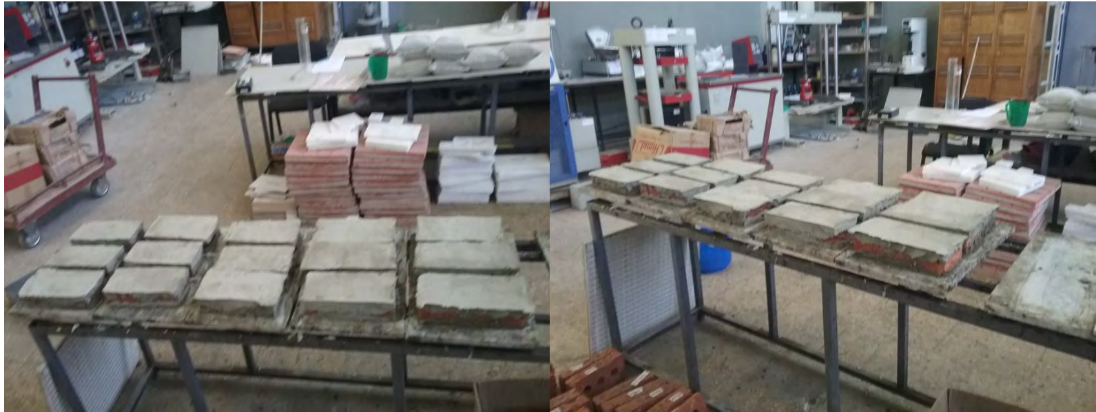
Picture B-11 Samples from Factory 1, 2 & 3 for Compressive strength test
