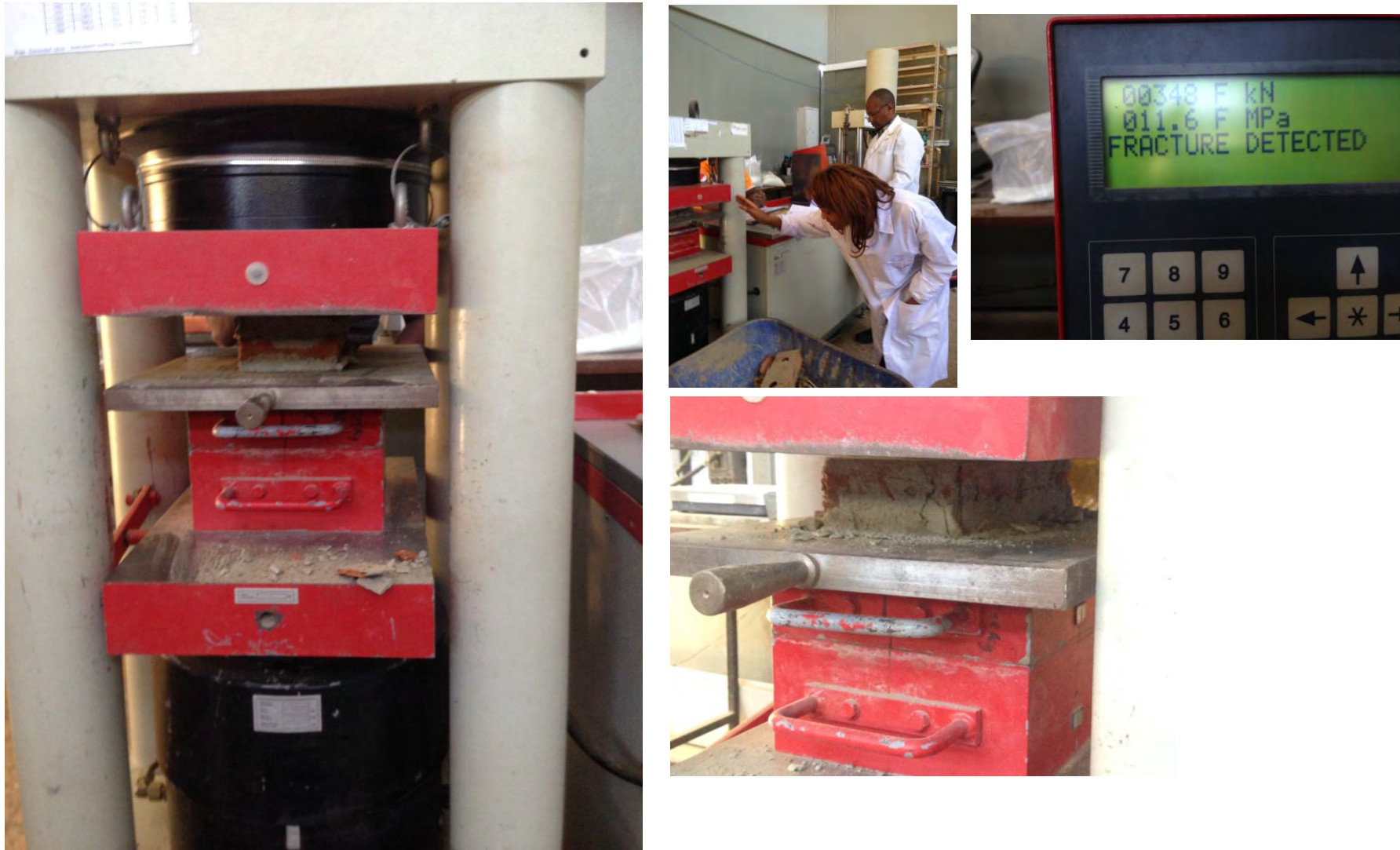
Picture B-12-Coping the brick surface for Compressive strength test
