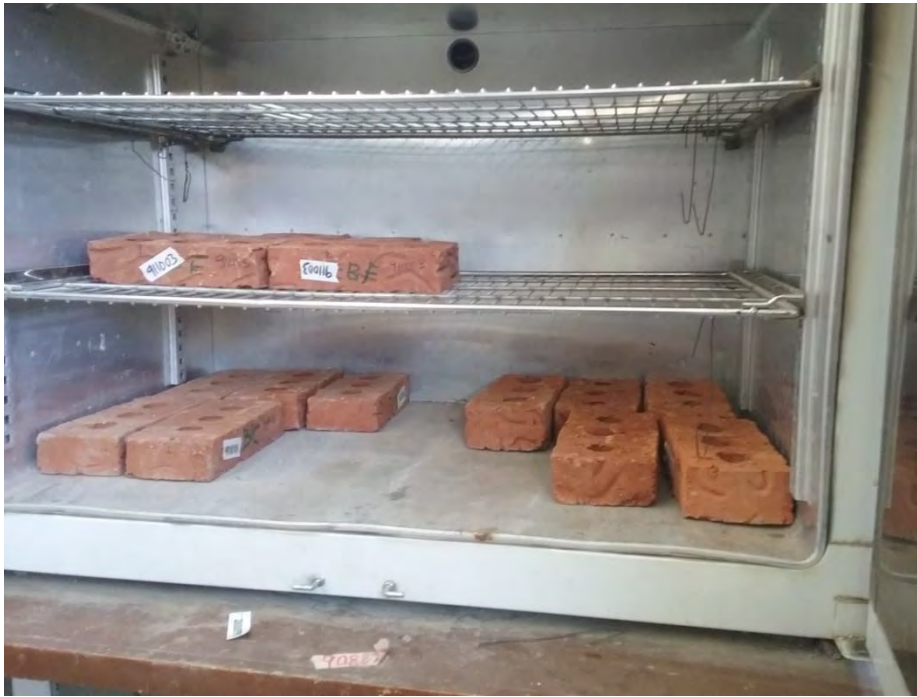
Picture B-15- 24hr oven drying for water absorption test - Step 1
