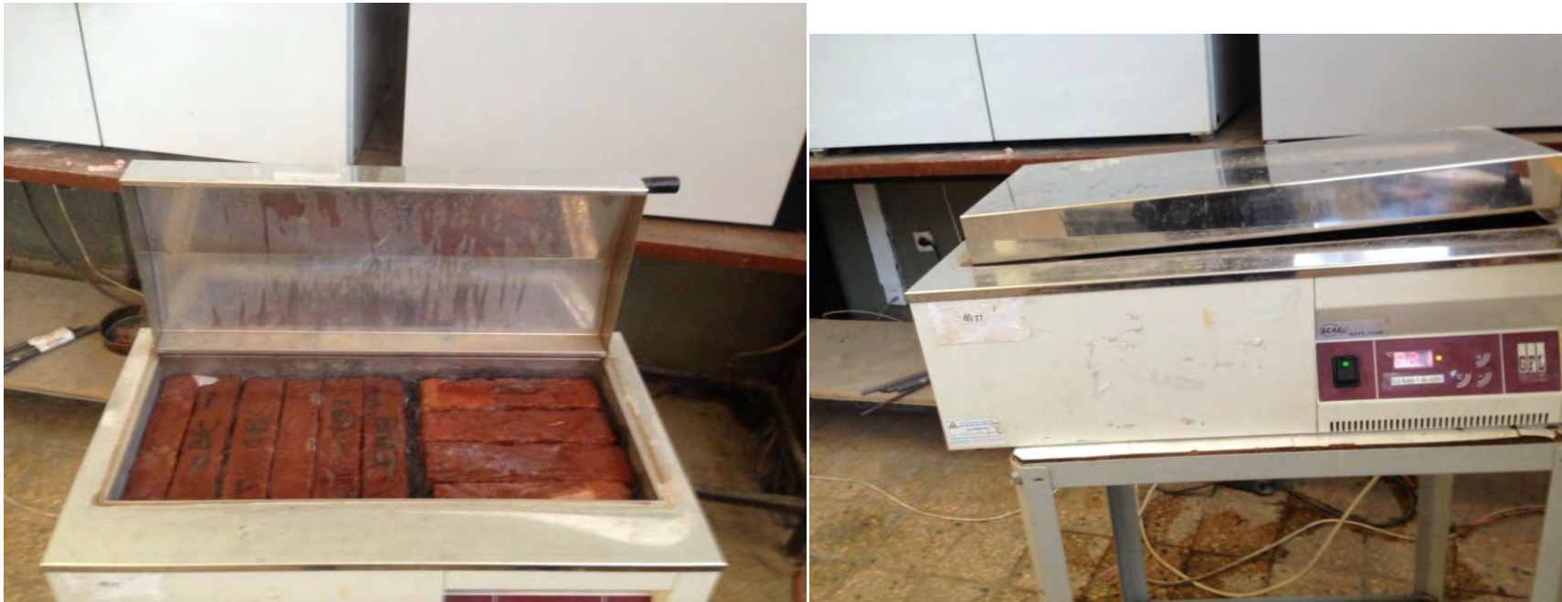
Picture B-17-24 hour boiling at 105° - Step-3
