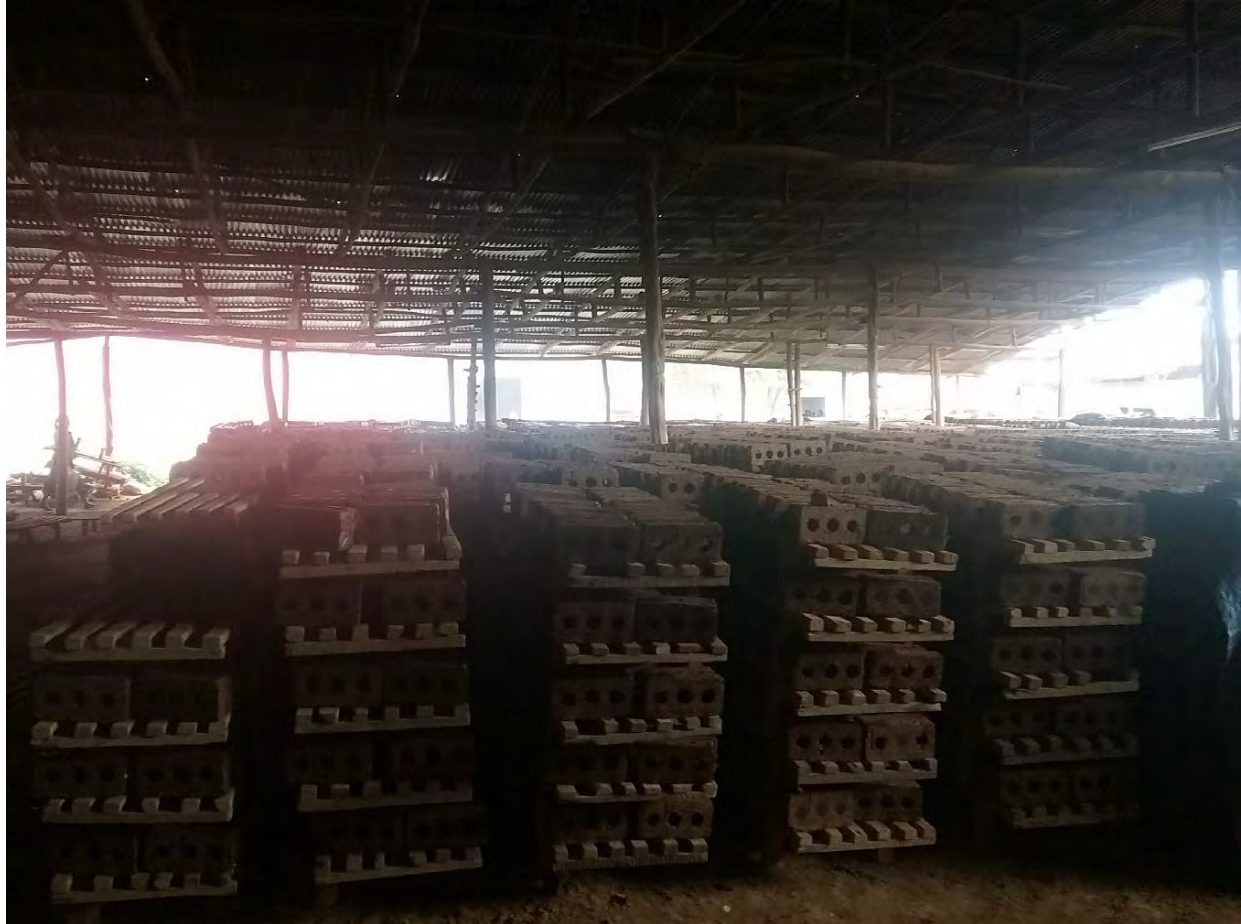
Picture B-2- Molded and cut clay bricks stay under shade to dry before firing - Ethio Bricks
