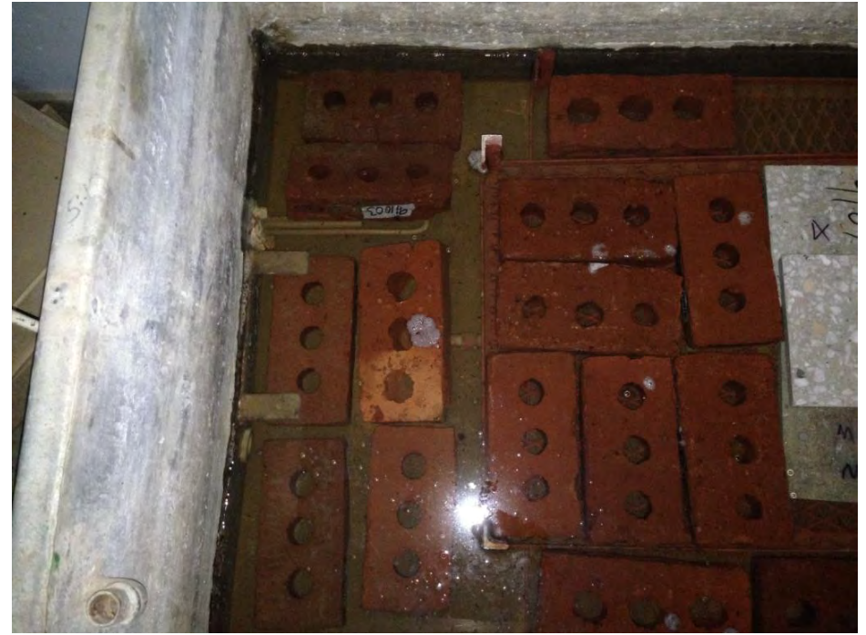
Picture B-16 - 24hr immersion in cold water for water absorption test - Step-2
