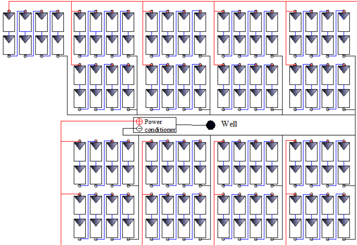
Figure 4.3 Block diagram for the arrangement of module in the array for well P1-BTW7
