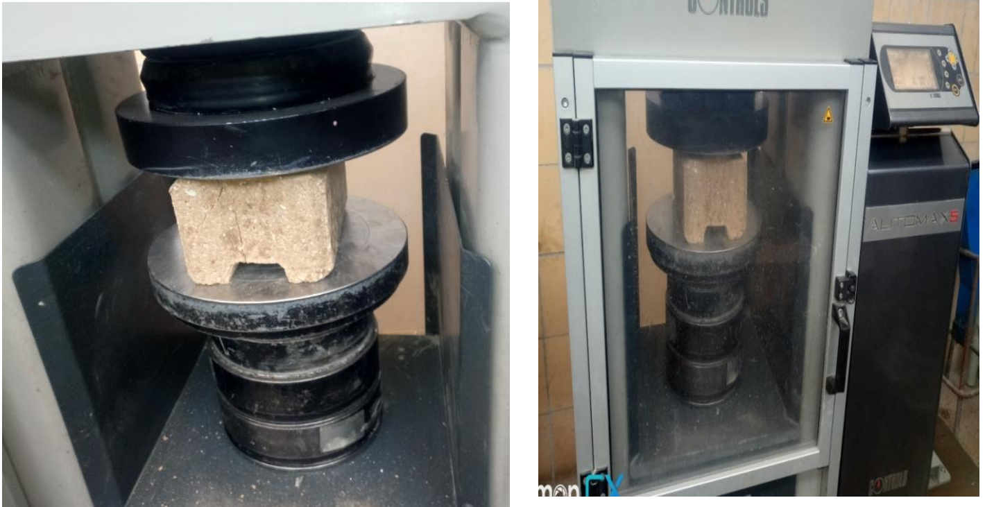
Figure4.7: Compressive strength testing of CSEB
