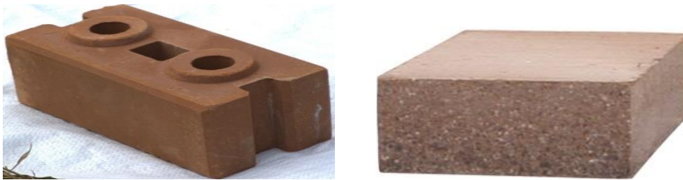
Figure2.1: Typical compressed earth block
