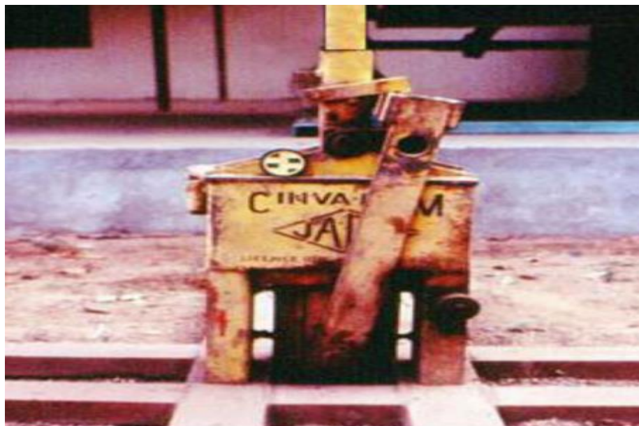
Figure2.2: The first original CINVA Ram Press Machine
