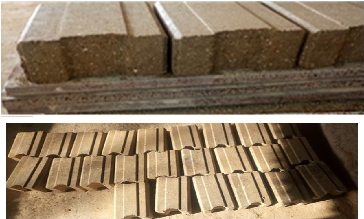
Figure3.6: Wet and Dry sample products of CSEB blocks
