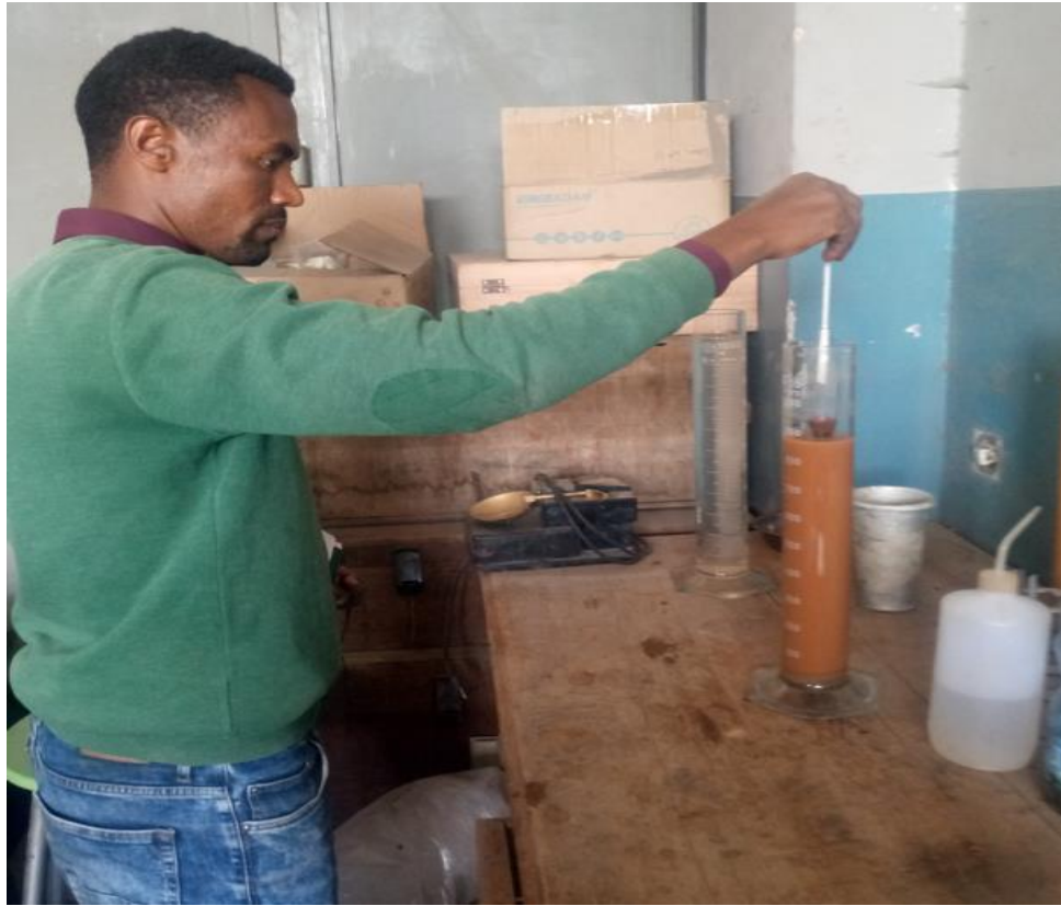
Figure3.2: Silt content determination of Soil
