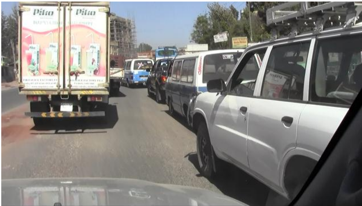
Figure 19: As there are no bus bays along the segment one lane is currently dedicated for loading and unloading passengers which results in long queue formation.
