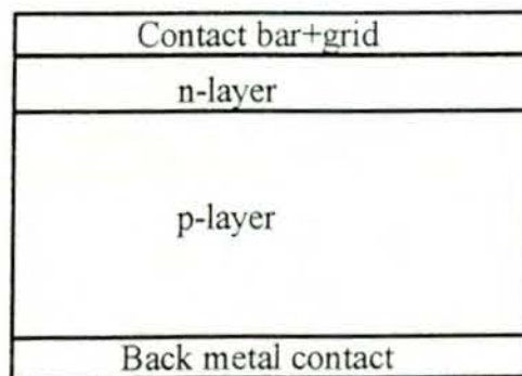
Figure 2.4 A p-n junction solar cell structure.
