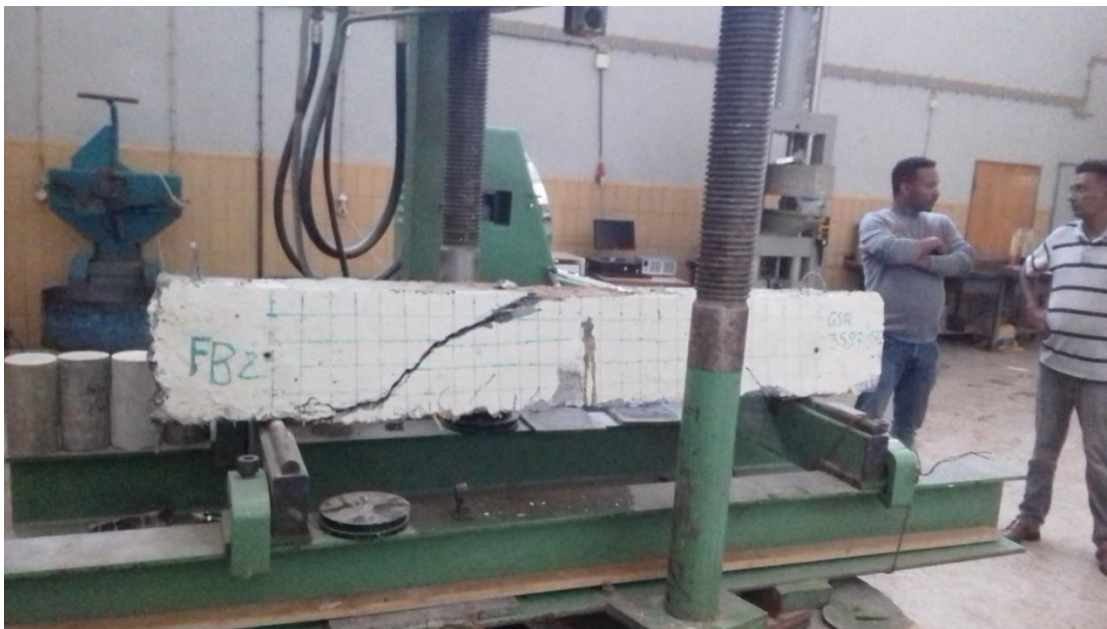
Figure 14: Fiber beam (FB-2)
