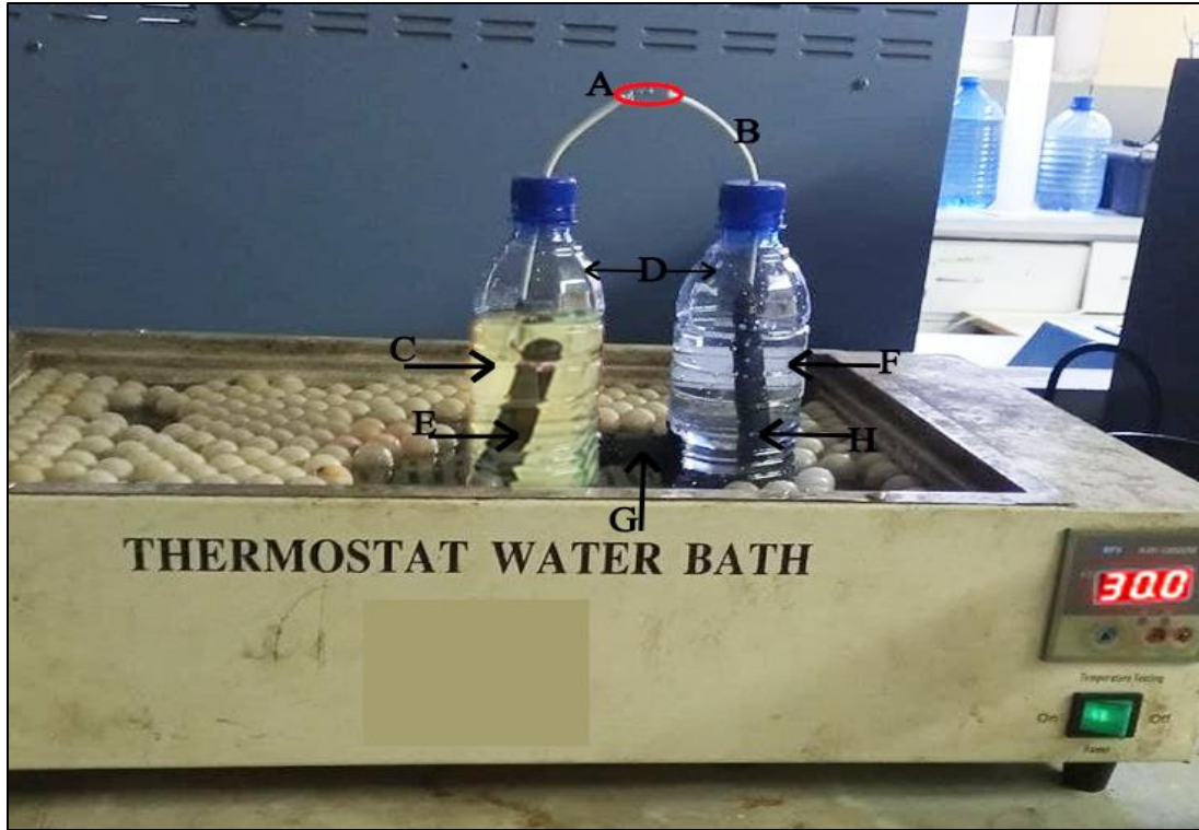
Figure 9: Full set up of Bio Electrochemical Fuel Cell used for Cr treatment
