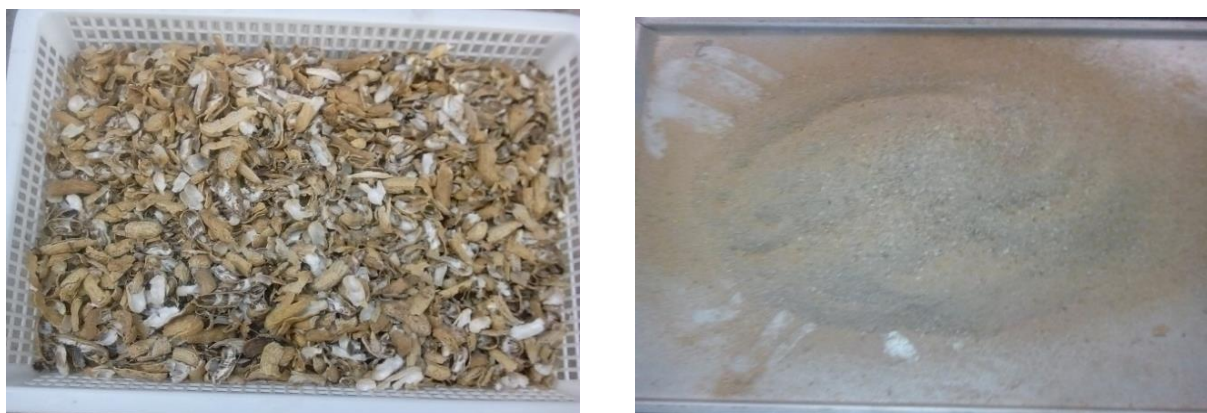
Figure 3.1: Preparation of peanut hull adsorbent. a) before grinding b) Peanut hull after grinding
