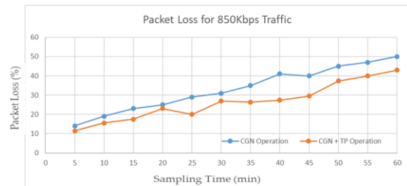
Fig. 5. Graph of packet loss for scenarios 1 and 2 of 850kbps traffic
