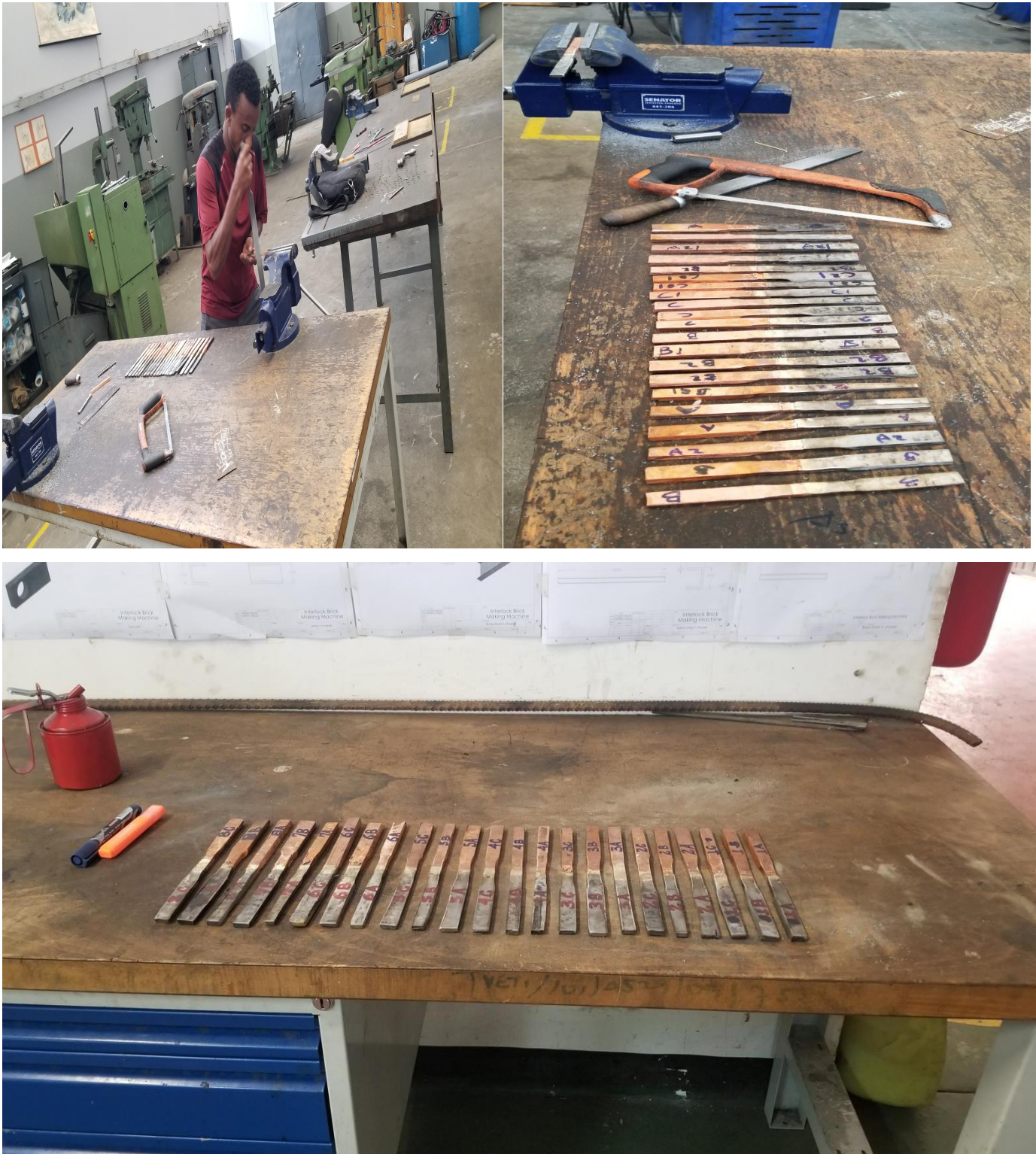
Figure 3.13 Ss -304L & Cc - 2.04 welding sample preparation for testing
