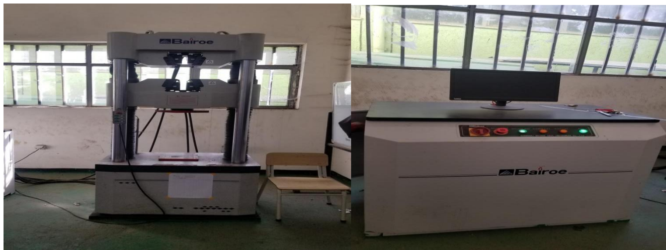
Figure 3. 15 Tensile test machine
