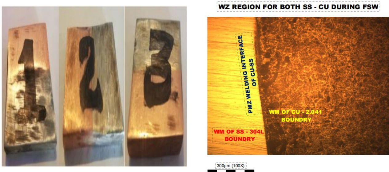
Figure 4.3 Optical micro-structural sample preparation and WZ observation
