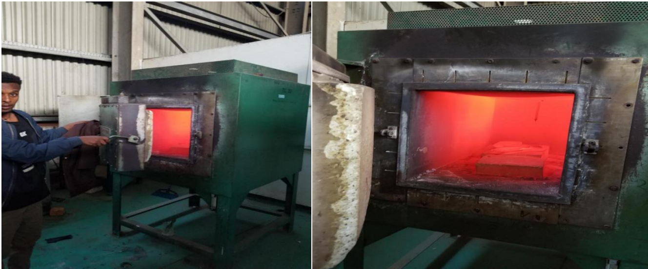
Figure 3.24 picture of annulling heat treatment in the furnace
