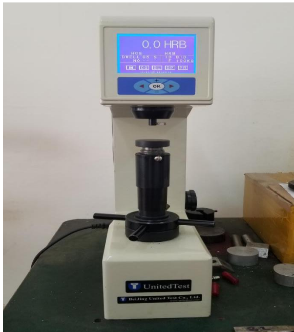
Figure 3.16 Rockwell hardness testing machine
