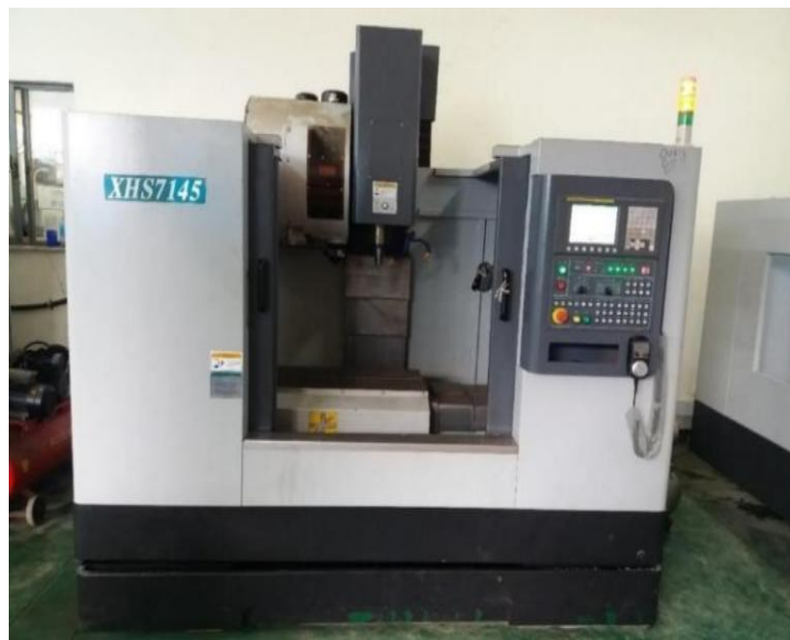
Figure 3.4 XHS7145 CNC milling machine or Vertical milling machine
