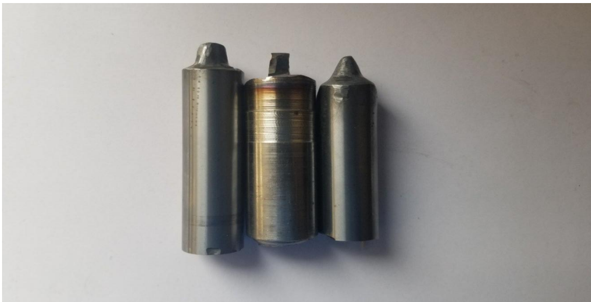
Figure 3. 9 Dimensions of welding tools 2D and 3D model for pin profiles, Actual image of tool Profiles: Square, Cylindrical and Conical
