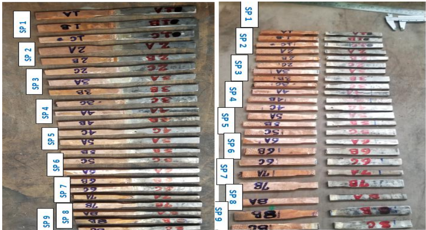
Figure 3.14 Before and after the tensile test
