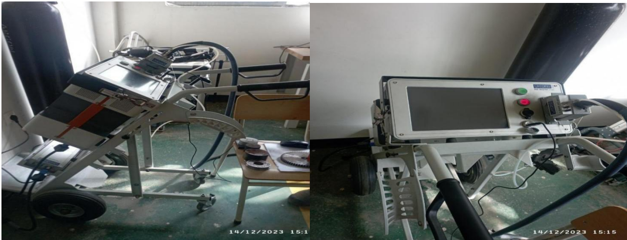
Figure 3.11 Spectrometer chemical composition of metals testing machine
