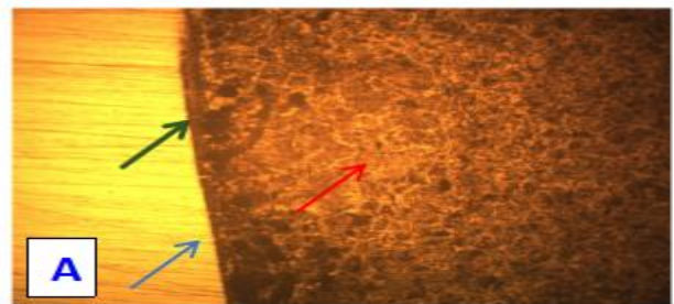
Sample 2 pure copper (CU-2.041) Heat affected zone
