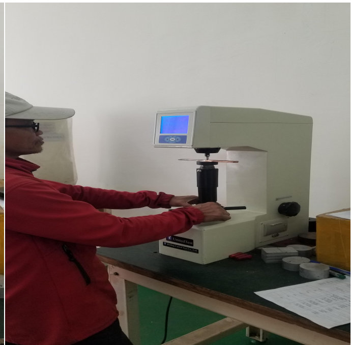
Figure 3.17 Hardness test of the specimen
