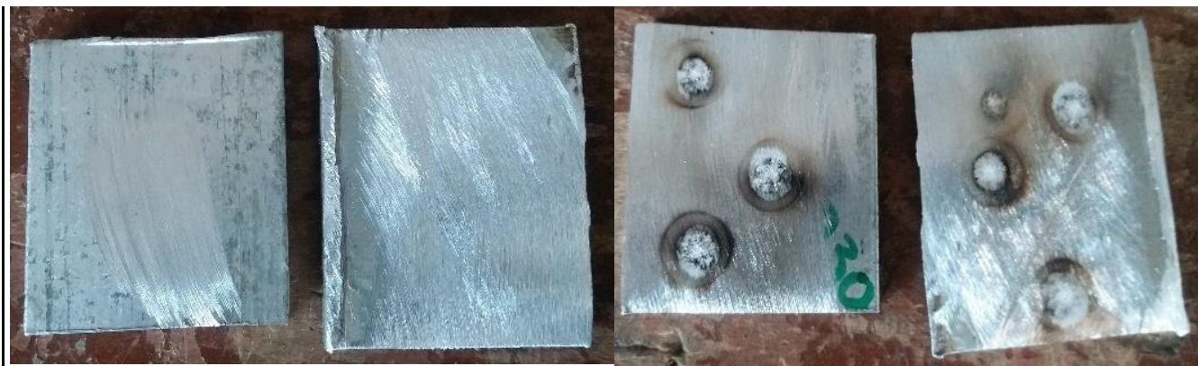
Figure 3.5 Sample of chemical composition of the metal was detected using SPECTROMAX
