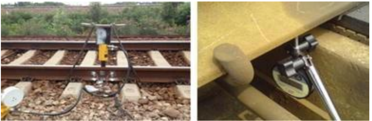
Figure 2-17: Jack-loading diagram and vertical rail deflection measurement
