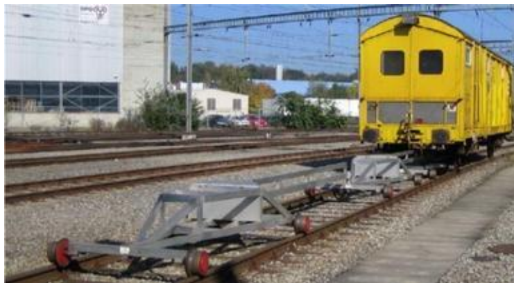
Figure 2-25: Track stiffness measurement vehicle of SBB
