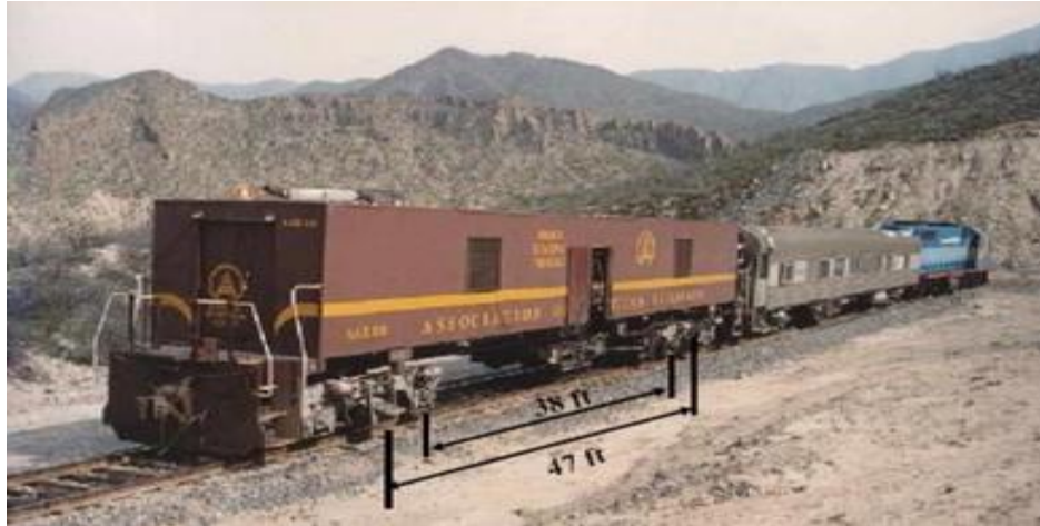
Figure 2-24: Track stiffness measurement vehicle of TTCI
