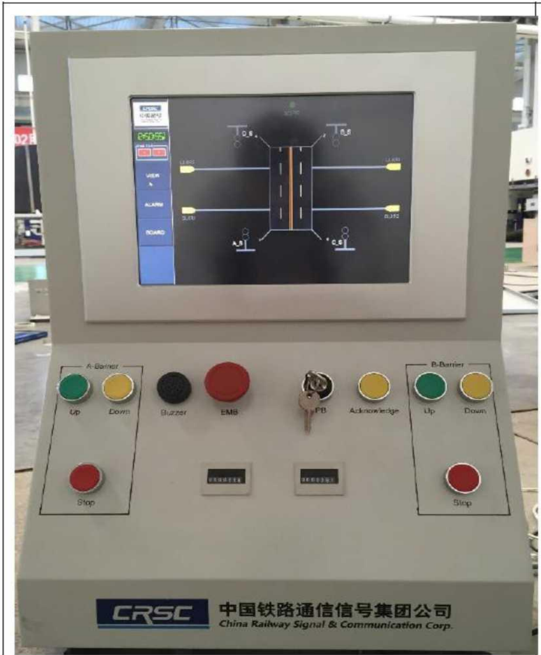
Figure2. 3: level crossing signaling around CMC area[21].
