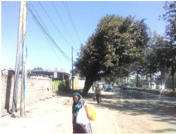
Picture 33: Struggle for space. Interaction between overhead power lines and street trees. (Source - Author)
