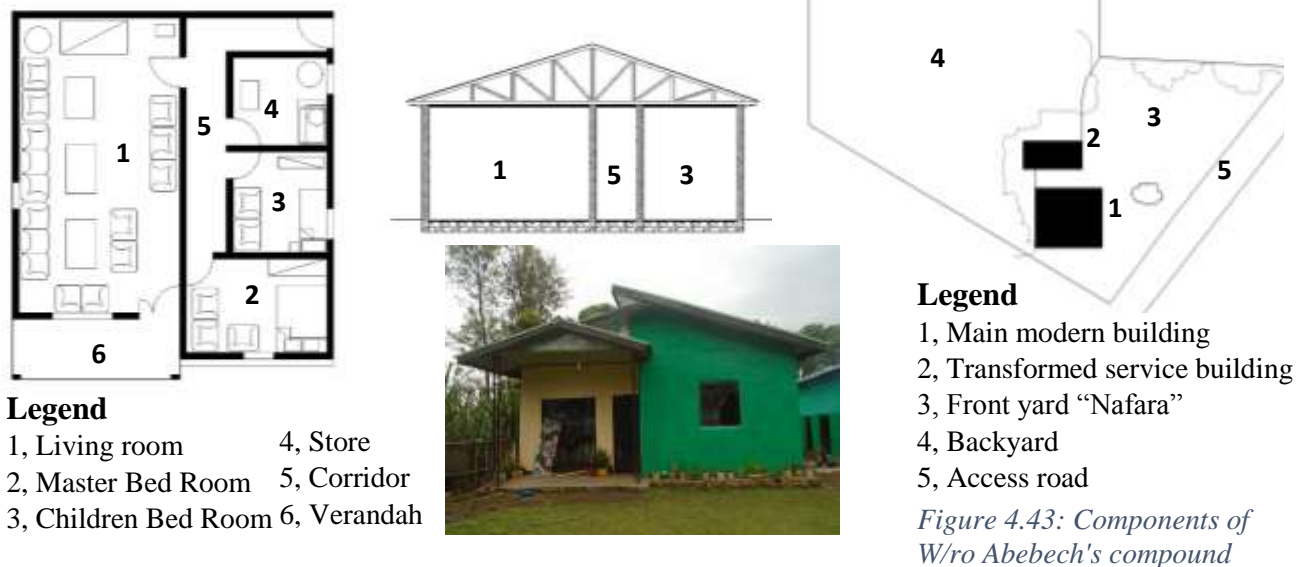
Figure 4.44: W/ro Abebech's modern main house plan, section and pic
