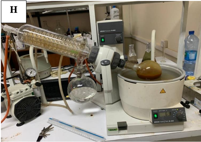
Picture of Rota Vapor (extraction equipment) (H) and Prepared extract for further drying in the oven (I)
