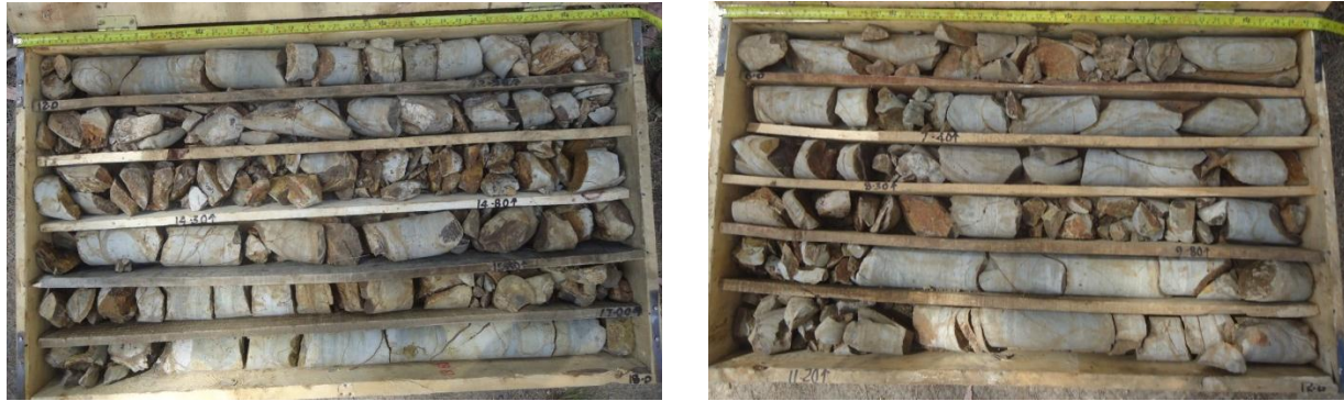
Plate 5.1: Photo showing the intensively fractured rock mass at the intake foundation
