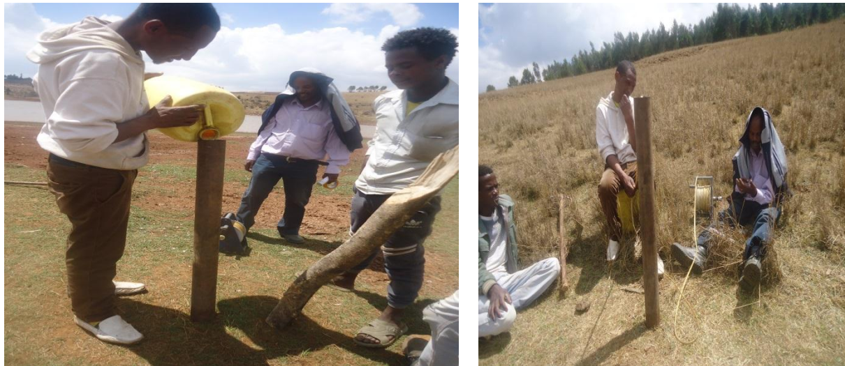
Plate 5.3: In situ infiltration tests in the reservoir area of the project area
