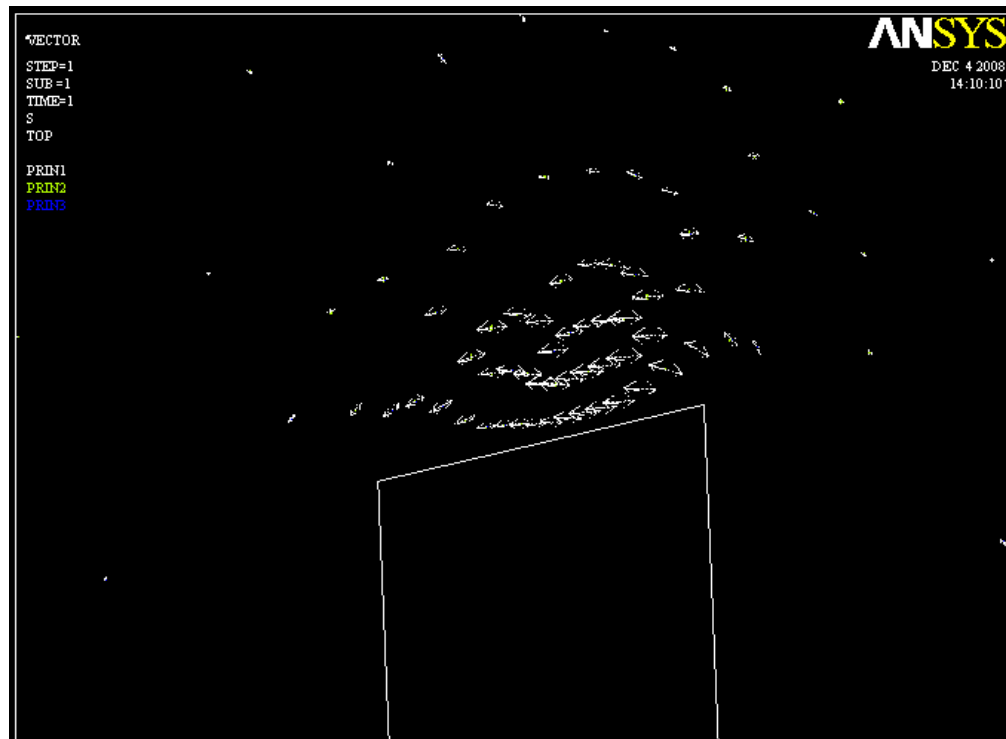
Figure 5.6(b) stress vector plot magnified at the crack tip
