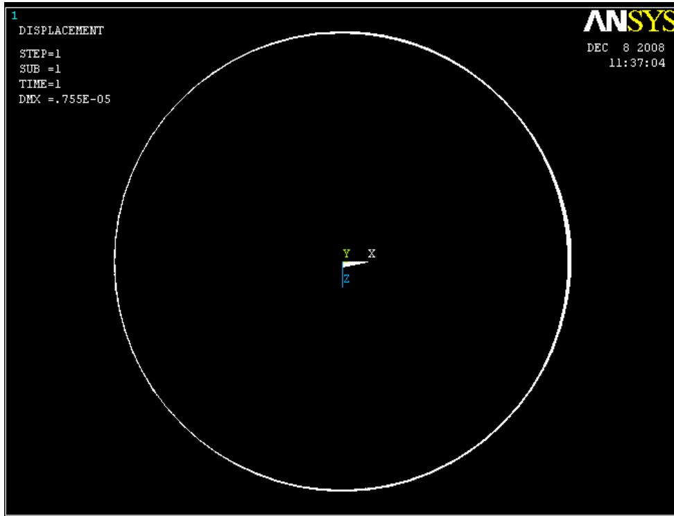
Figure 6.1 c) Deformed shape of isotropic cylindrical shell towards crack side
