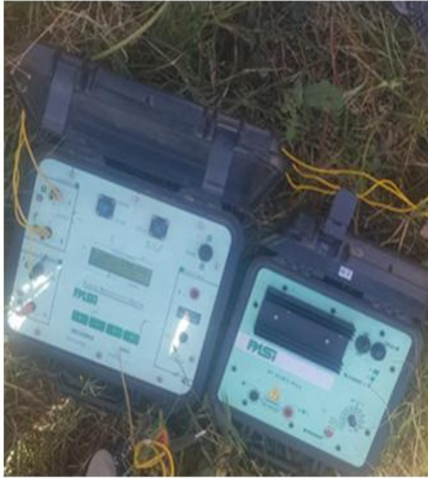
Figure 4. 51Data acquisition by PASI-GL16 Earth resistivity Meter and P100-N x Energizer units
