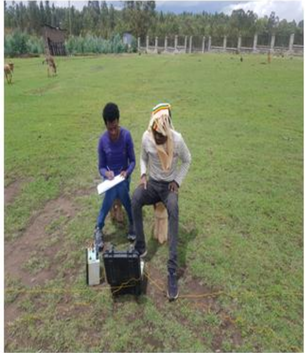
Figure 4. 51Data acquisition by PASI-GL16 Earth resistivity Meter and P100-N x Energizer units
