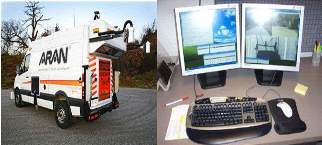
Figure 7: Pavement inspection vehicle ARAN [13]
