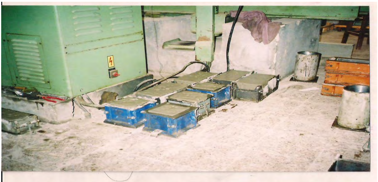
Photo 6: Concrete specimens after casting
