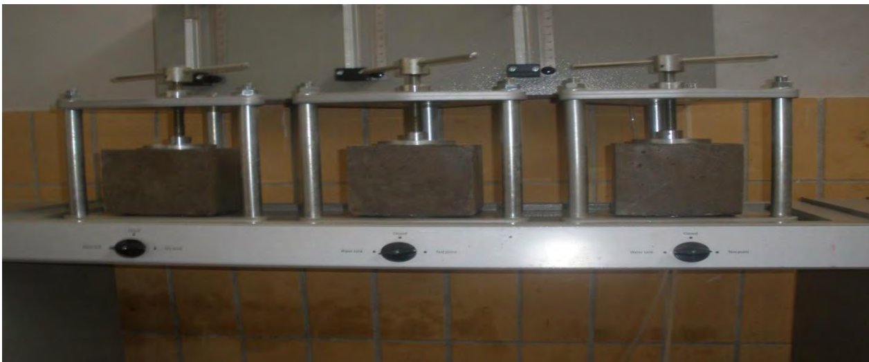
Fig 5.2: Permeability apparatus with the test cubes assembled on it
