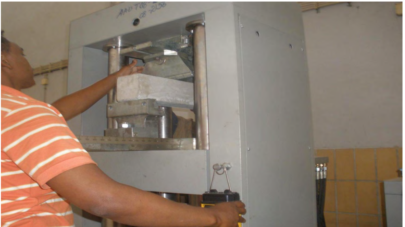
Photo 10: Concrete specimen during flexural strength test
