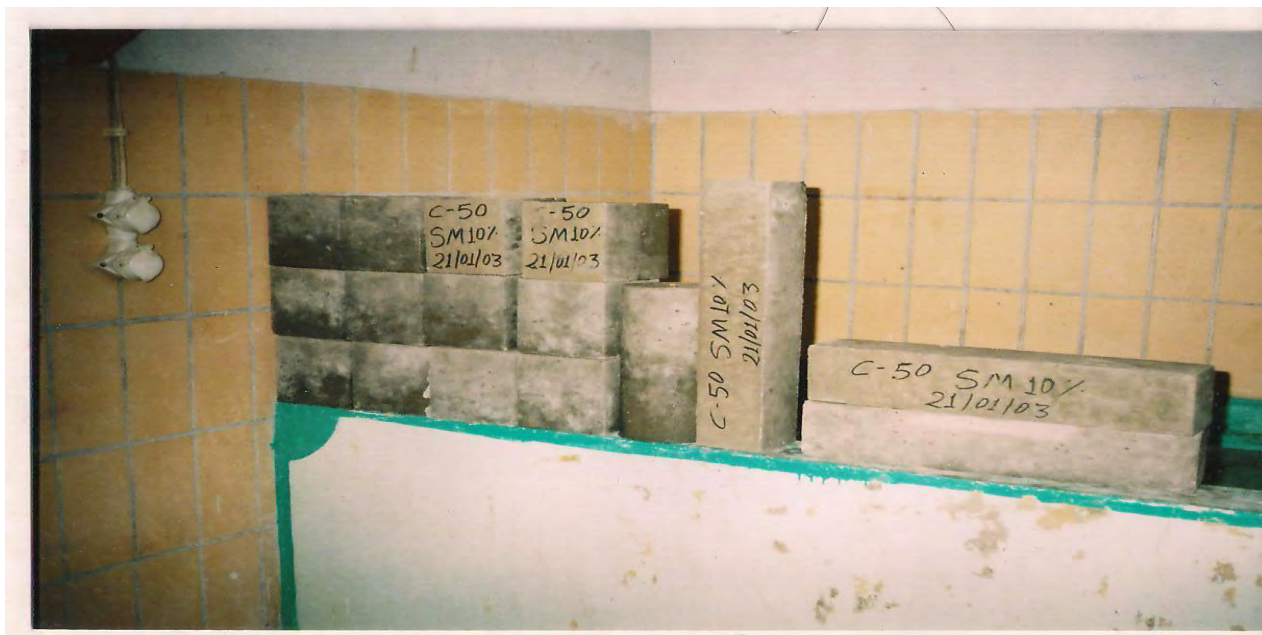
Photo 8: Concrete specimens arranged for test
