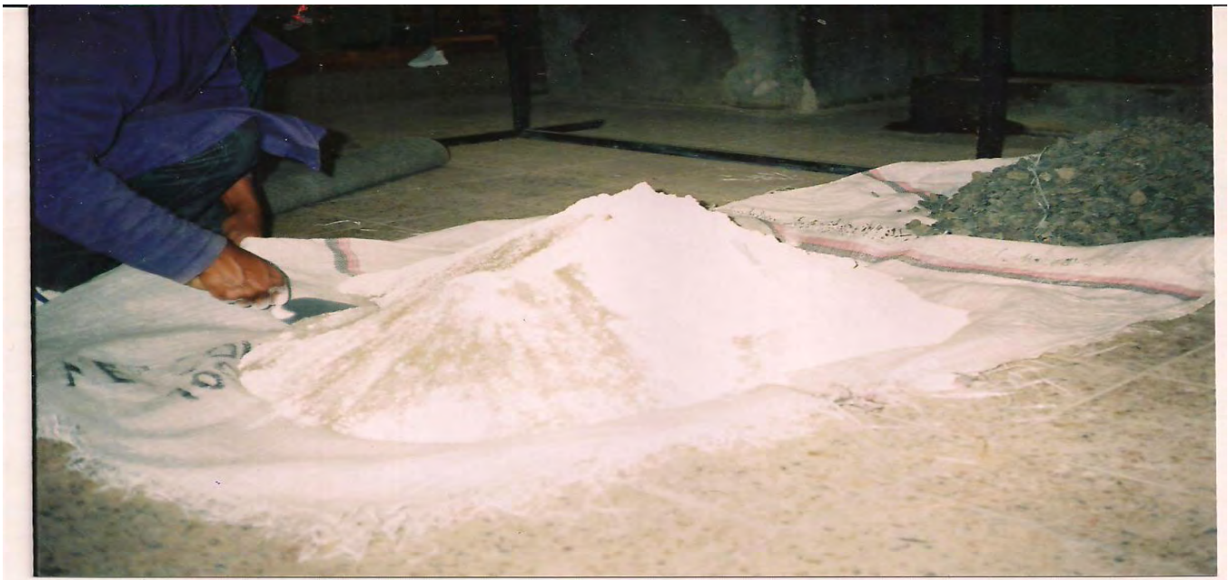
Photo 2: Batching and blending of marble waste powder with sand
