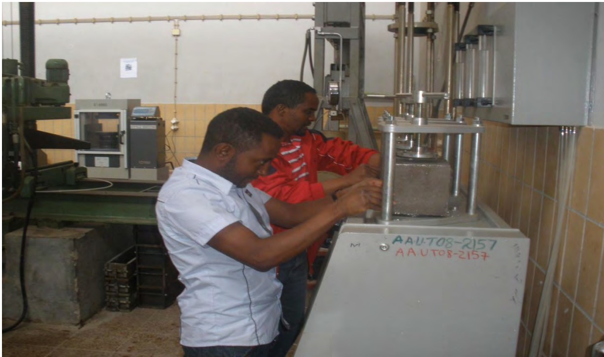
Photo 12: Arranging concrete specimens for water permeability test
