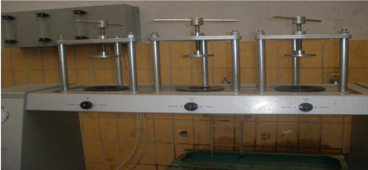
Photo 11: Water permeability testing apparatus
